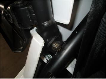
2. With the door in the open position, tilt the front of the door down and pull the upper mounting bracket out from the b-pillar. Then pull the lower mounting bracket out from the plastic trim.
