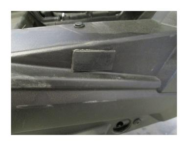
9. Place an adhesive rubber strip (Item 15) where the door meets the plastic trim at the lower front corner. This will eliminate any unwanted audible vibration between the door and plastic trim.
