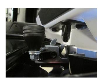
12. Take the door limit strap (Item 6 & 7), loop it around the chassis tube, and shoot it through the slider bracket as shown below. Then take the M6 button head flanged bolt (Item 8) and the M6 acorn nut (Item 9) and fasten the other end of the door limit strap to the tab on the door frame.
