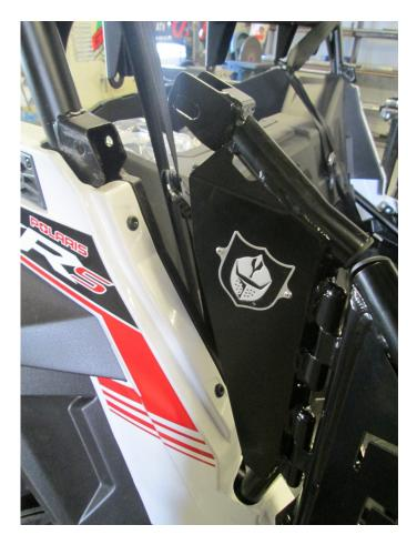
4. Take your Proarmor door and insert the lower mounting bracket through the plastic trim. Then line up the upper mounting bracket to the b-pillar.
