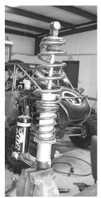
4. Compress the spring and remove the retaining collar from the shock.
