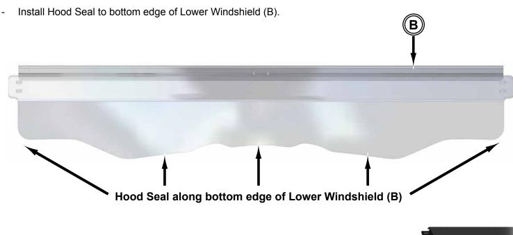
To ease installation, soak Seal in hot water before cutting or installing to increase flexibility.
