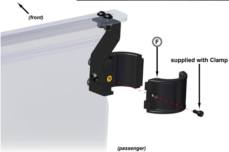
Install Handle and Support, part of Latch Assembly (D), to Upper Windshield (A) with hardware shown.
