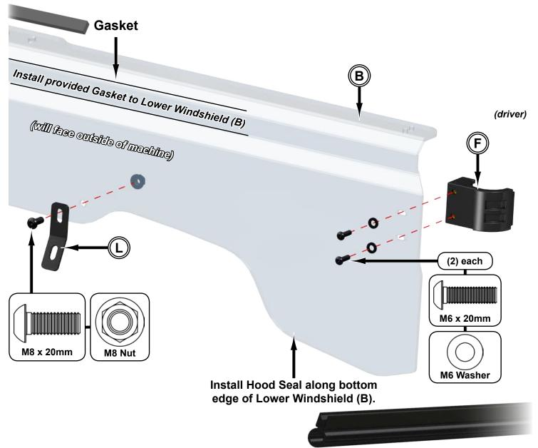
To ease installation, soak Seal in hot water before cutting or installing to increase flexibility.
