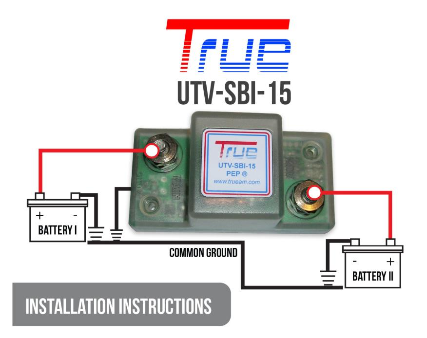
FYI: The SBI is designed ambidextrous so it cannot be installed backwards. Either stud can be connected to either battery's positive terminal.
