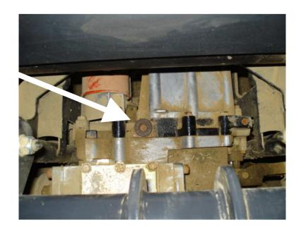
2) Clean all dirt and debris from area to prevent any contamination. Remove plug with 10mm hex wrench.
