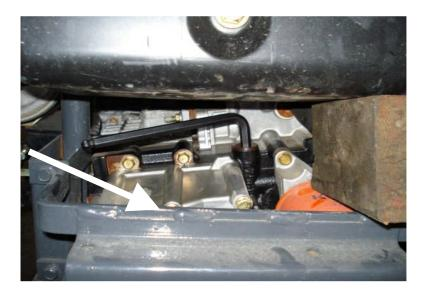
3) Using a magnet, remove spring and relief valve.
