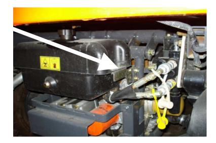
1a) On RTV1100 units, raise the bed and locate the relief valve plug by looking between the muffler and frame cross member.
