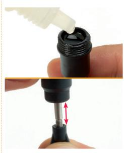
When the oil level nears the top of the body, move the shaft slowly up and down so that the oil spreads throughout the assembly and displaces any air below the piston. Repeat this process until no more bubbles appear.
