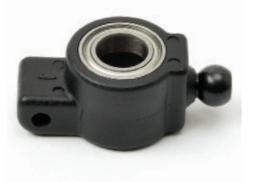
Turn the hub carrier over and repeat Steps 06 and 07 with the second ball bearing.
