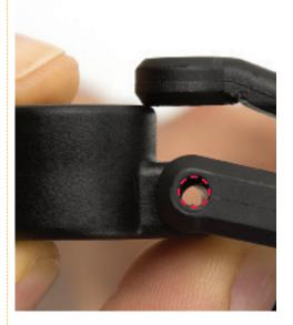
Make sure the holes in the carrier and the lower wishbone are correctly aligned, as shown by the circle.
