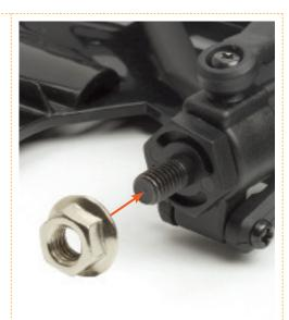
13 Fit the 6mm flange nut over the tip of the wheel shaft.
