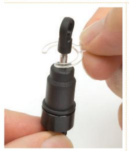
13 Holding the shock absorber body as shown, slide the spring spacer over the shaft until it rests against the ridge at the base.
