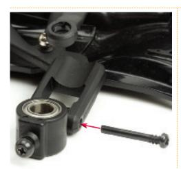
Place the screw pin into the righthand side of the lower wishbone, and push it through until its tip is visible at the left-hand side.
