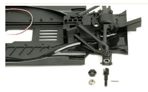
Position your RB7 on your work surface as shown, facing to the left, with the new parts in front of the left rear hub carrier and suspension. This will give you an idea of where the parts will fit.
