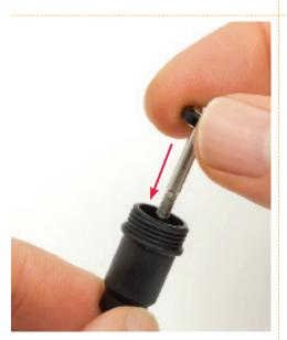
Remove the pre-fitted end cap from the shock absorber body so that the threaded section is visible. Then, holding the body as shown, push the shaft into the case until it protrudes through the hole at the other end (see Step 05).
