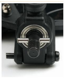
Adjust the pin so that equal lengths of it protrude from each side of the shaft.
