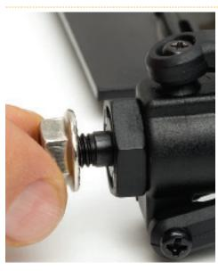
Turn the flange nut clockwise by hand to tighten it until it begins to turn the wheel shaft.
