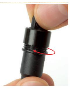
Wipe away any excess oil using a cloth, then take the shock absorber cap and top assembly and screw it onto the threaded section of the body. Turn it in the direction of the arrow until tight.
