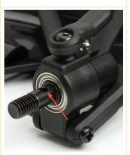
Push the shaft through the hub carrier until the hole near the threaded end is fully visible (arrowed).
