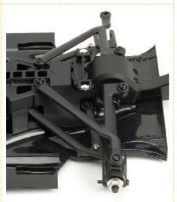
Check that the ball is properly fitted within the hole in the wishbone and that your assembly looks like this. The rear left suspension system is now nearly complete.
