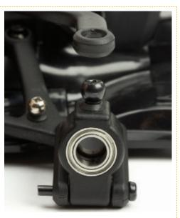
Check that the hub carrier is able to move up and down freely. If it sticks, loosen the screw pin by a quarter turn. Position the carrier vertically, as shown in the photo.
