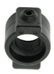
Pamiliarise yourself with the rear hub carrier. The circular recesses will house the ball bearings, and the hole in the top and projection at the bottom will connect the part to the two wishbones.
