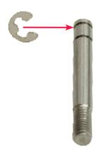
Using needle-nose pliers, clip one of the E-rings into the first groove on the unthreaded end of the shock absorber shaft.
