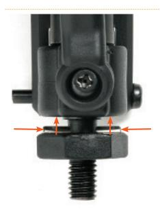
Push the drive washer towards the hub carrier and seat the pin within the groove.
