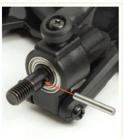
7 Insert the pin into the hole.
