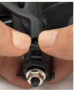
Re-attach the left rear wishbone and hub carrier by lining up the ball-headed screw with its socket and pushing the two together firmly until the ball clicks into place.
