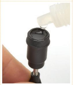
When any air bubbles are gone, carefully fill the case to the brim with shock absorber oil. Make sure that no more bubbles are formed when you add the oil, and that no oil overflows onto the outside of the body.
