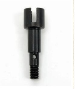
2 At one end of the wheel shaft there is a slot, and near the threaded end there is a hole through which the pin will be inserted.
