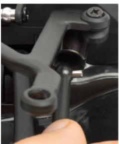
2 Place one end of the driveshaft into the differential shaft, as shown. The metal pin should fit into the slots in the differential shaft.
