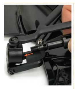
Hold the wheel shaft with the threaded end pointing away from the chassis, and push it through the left rear hub carrier from the inside.
