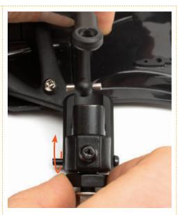
Holding the driveshaft in place within the differential shaft, position the hub carrier so that the metal pin at the outside end of the driveshaft lines up with the corresponding slots in the inside of the wheel shaft. Then tilt the hub carrier up so that the driveshaft fits into the wheel shaft.
