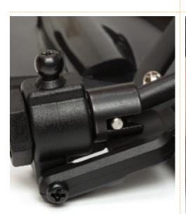
Your assembly should now look like this. Make sure that both ends of the driveshaft are sitting within the slots in both the differential and wheel shafts.
