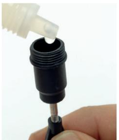
Holding the shock absorber body upright and with the shock shaft fully extended, carefully begin to pour in the shock absorber oil you received with Stage 4 – there should be enough left over from the work you did on the front shocks.
