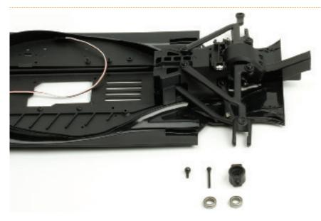
Position your RB7 on your work surface as shown, facing to the left with the new parts in front of the left rear suspension. The hub carrier will connect the upper and lower wishbones, so that the rear wheel shaft and eventually the rear wheel can be fitted.
