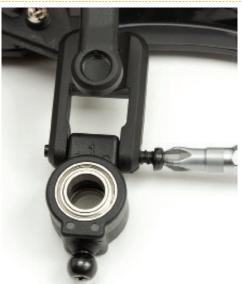
Tighten the screw pin with a screwdriver.
