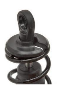
The spring should fit comfortably within the ridge on the underside of the lower spring holder, as shown.
