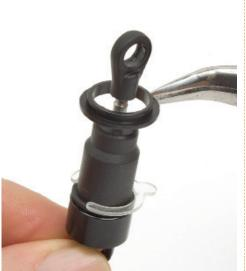
Next, use needle-nose pliers to fit the upper spring holder over the body and slide it down so that it rests on top of the spring spacer.
