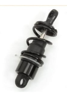
This session is now complete, and your assembly should look like this. The plastic spring spacer is designed so that it can be removed without having to take the shock body apart.
