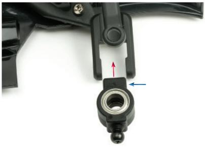
Place the hub carrier assembly flat on your work surface, positioned as shown in the photo for Step 08. Then slide it in between the arms of the lower wishbone (red arrow), making sure that the hole through the carrier's lower section (see blue arrow) is perfectly aligned with those on the ends of the wishbone's arms.
