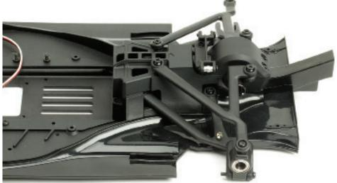
This stage of assembly is complete, and your model should look like this, with the hub carrier connecting the two rear wishbones, ready to accommodate the left rear wheel shaft and wheel.
