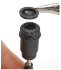
Hold the diaphragm with needlenose pliers so that the domed side is facing downwards. Slowly place it on top of the body, taking care to avoid creating air pockets in the oil.
