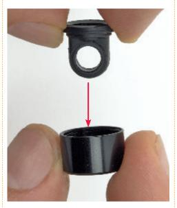
Holding the cap as shown, push the shock absorber top into the hole in it (indicated by the red arrow) as far as it will go.
