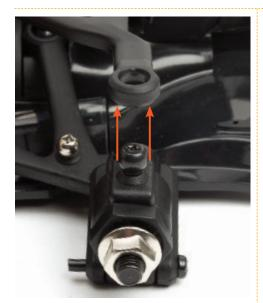
Place your RB7 racer on your work surface, facing to the left. Carefully pull the left rear wishbone and hub carrier apart, so that the ballheaded screw on the top of the carrier comes out of the hole in the wishbone.
