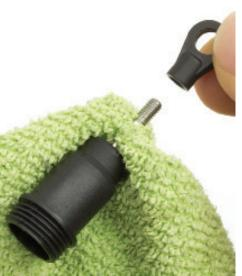
O5 Cover the threaded section of the shaft with a cloth to protect it from scratches, then use needle-nose pliers to pull the shaft as far out of the case as it will go. Hold the shaft in place, then screw the ball end on a little way.
