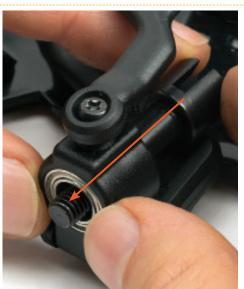
4 Slide the shaft through the hub carrier until the threaded end protrudes.
