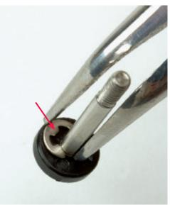
O3 Clip the second E-ring into the other groove. The shock piston is now sandwiched between the two rings.
