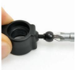
Tighten the ball-headed screw with a screwdriver, making sure not to overtighten it as that may damage it.
