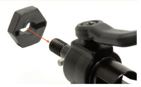
1 OSlide the drive washer over the end of the wheel shaft, with the groove facing towards the pin that you fitted in Step 07.
