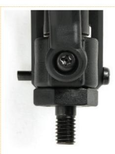
12 Push the drive washer up against the hub carrier, as shown in the photo.
