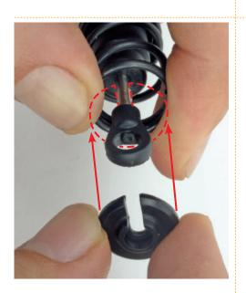
Hold the body assembly in one hand and pull back the spring, as shown. Place the lower spring holder in the gap on the shaft between the spring and ball end. Gently release the spring so that it comes to rest as shown in Step 17.
