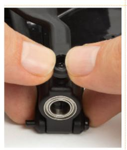
Position the upper wishbone so that the socket at the end of the longer control arm is sitting on top of the ball-headed screw. Press down on the control arm until the part clicks into place, with the ball inside the socket.
