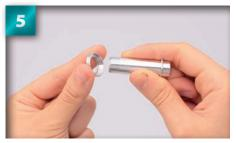
Remove the servo saver adjuster from the servo saver shaft.
