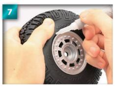
Ease the sidewall back a little, creating a small gap between the tire and the wheel rim, then squeeze a small amount of instant adhesive into the gap. See the Tip box on the right for the recommended technique for applying the glue.
