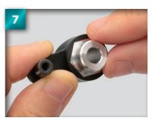
Engage the hexagonal projection with the corresponding recess in the hole of the servo saver, as shown.
