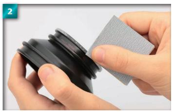
While waiting for the tire to dry, use wet and dry paper to remove the paint from the rims of the wheel (which was provided in Stage 1). This will help with adhesion.
