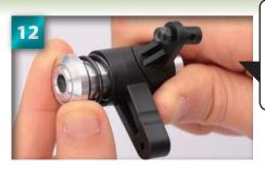
Use the servo saver adjuster to push the spring in, and screw the adjuster onto the end of the shaft.
