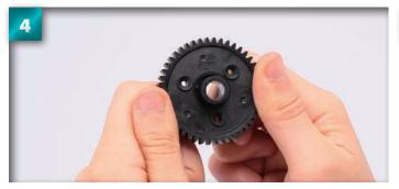
Push the gear holder and gear together firmly until there are no gaps between them.
