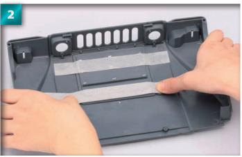
Secure the radiator cover with masking tape to prevent it from moving.
