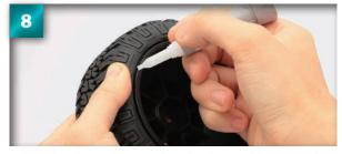
When the glue is dry, turn the wheel assembly over and repeat Step 7 for the other side.
