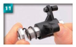
Place the servo saver adjuster onto the servo saver spring.
