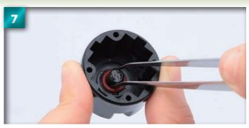
Push the O-ring down the joint until it sits in the recess that you greased in Step 2.
