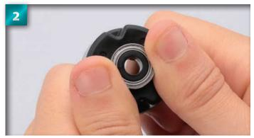
Press the bearing firmly into position on the projection. Make sure the bearing is aligned with the case.
