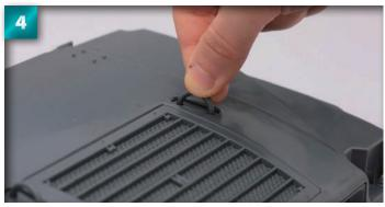
Fit the second hook on the other side of the hood. If the hooks are inserted too forcefully, the temporarily fitted radiator cover may come loose, so support the cover from behind while fitting the hooks.
