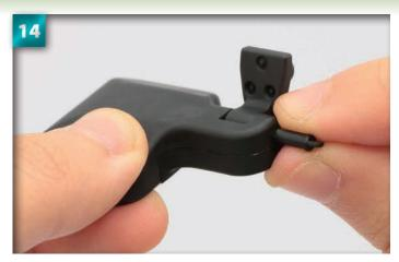
Insert the side mirror pin into the hole in the bottom of the side mirror cover.
