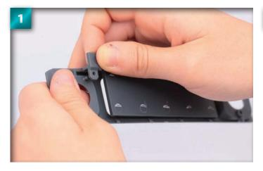
Carefully remove the front grill mesh from the front grill, temporarily assembled in the previous stage.
