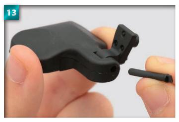
Locate the hole in the bottom of the side mirror cover into which the side mirror pin fits.
