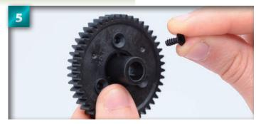
Insert one of the screws into one of the countersunk holes on the front of the gear.
