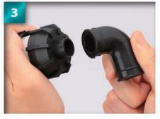
Fit the air pipe onto the air filter base. If it is difficult to insert, use a little wet and dry paper on the inside of the pipe.
