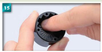
Push the bevel gear down onto the joint until the pin slots into the groove.
