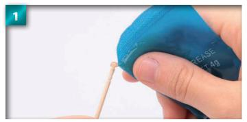
Cut a corner from the grease bag and place a small amount of grease onto the end of a toothpick, or similar.
