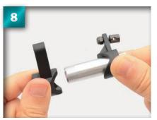
Hold the servo saver shaft and insert it into the servo saver lower arm. The stopper should be oriented as shown in the photograph.
