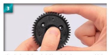
Align the three holes in the holder with the three countersunk holes on the gear.
