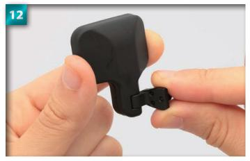
Insert the second side mirror arm into the hole in the base of the mirror cover.
