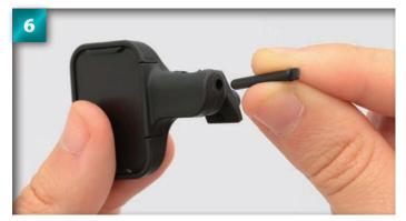
Locate the hole in the bottom of the side mirror cover into which the side mirror pin fits.
