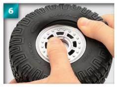
Turn the wheel assembly over and position the other side of the tire into the groove on the other side of the wheel.
