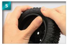
Working around the wheel, pull the shoulder of the tire back slightly to help ease it into the groove on the inside of the rim.
