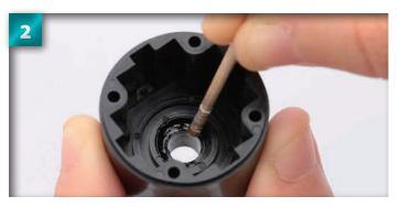
Apply some grease to the recess in the center of the inside of the differential case.
