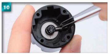
Insert the 2.5  $\times$  10.3mm pin into the hole in the joint, just above the shim.
