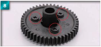
At this point in the assembly there should be 1mm gaps between the heads of the screws (circled in red) and the front face of the gear.
