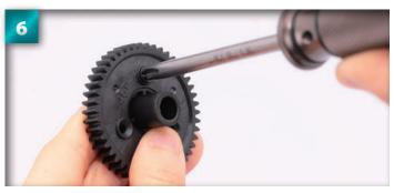
Use a size 2 Phillips screwdriver to tighten the screw. Do not tighten the screw fully: leave about 1mm between the screw head and the front face of the gear.
