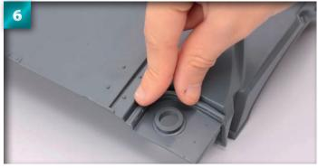
Align the pins on the underside of the gasket with the holes in the hood.
