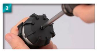
Insert the  $3 \times 10$ mm self-tapping screw into the hole in the middle of the air filter cover and tighten slowly with a size 2 Phillips screwdriver.
