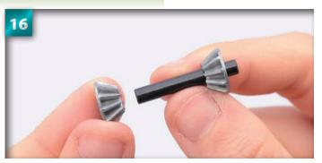
Slide a 10T bevel gear onto each end of the bevel gear shaft, as shown.
