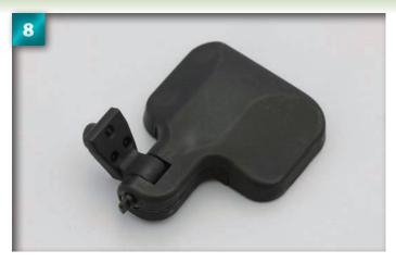
The left side mirror is now complete. If there are any burrs around the parts, carefully remove them, using a knife.
