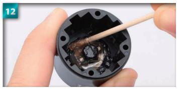
Smear some extra grease around the shim and the joint.
