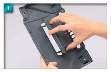
Fit the radiator cover into the opening in the center of the hood, from the underside.
