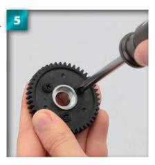
Place the first 1480 ball bearing into the space in the centre gear, as arrowed. It does not matter which way round the bearing goes.
