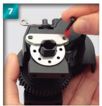
Place the first 3 × 12mm binding-head screw provided in Stage 39 through the holes on the right of the brake pads and callipers, and into the hole in the gear mount beneath.
