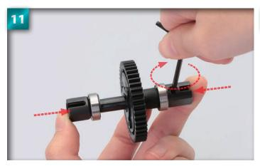
Applying pressure with your hands to keep the parts tight to each other, tighten the set screw firmly with the Allen key.
