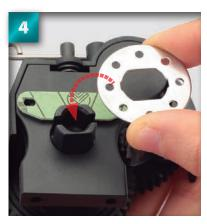
Fit the brake disc over the protruding cup joint.
