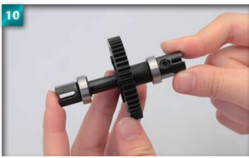
Push the cup joint down so that it rests against the gear. If it is difficult to push it, loosen the set screw a little.
