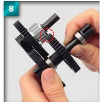
Adjust until the teeth of the centre gear engage fully with those of the main gear (circled). Make sure not to force the parts, as this may damage the teeth. Once engaged, ensure the centre gear is sitting straight.
