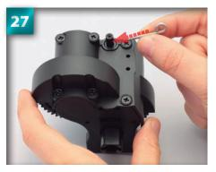
Push the brake cam rod through the hole in the shaft of the brake cam protruding from the gear cover.
