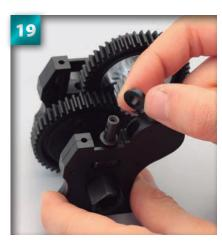
Press the brake collar down so that it rest on the upper edge of the gear mount.
