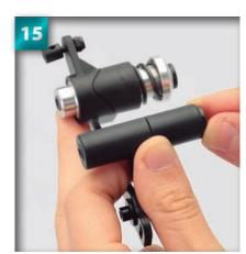
Pull the servo savers apart gently and place the assembly directly behind the front bulkhead from the rear.
