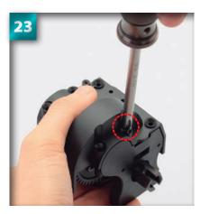
Next, repeat for the next three circled holes. Do not fully tighten the screws at this stage.
