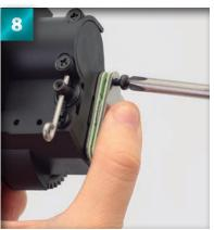
Holding the parts in place, gently tighten the screw, but stop before the head touches the outermost calliper.
