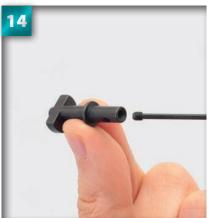
Hold the brake cam level, as shown, and carefully insert the set screw. Make sure that the set screw is in perfectly straight, then tighten by two rotations.
