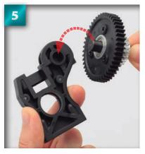
Insert the tip of the main gear shaft into the hole in the underside of the centre gear mount back, following the arrow.
