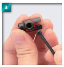
Place the set screw into the threaded hole in the side of the main shaft cup joint (circled). Do this immediately, before the thread-locking agent or adhesive dries.
