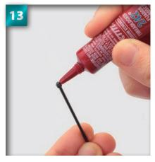
Place the 3 × 3mm set screw onto the tip of the Allen key, and apply a little thread-locking agent (or rubber-based adhesive).
