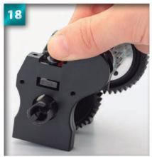
The short side of the cam should be visible in the rectangular hole from the outside of the gear mount.
