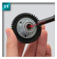
Place the longer end of the main gear shaft into the front of the centre and main gear assembly, as shown by the arrow.
