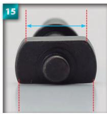
Position the gear mount assembly on your work surface, as shown, then carefully place the brake cam into the arrowed slot, with the short side of the cam facing you.
