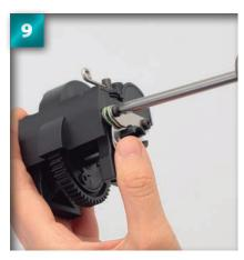
Tighten the second 3 × 12mm binding-head screw (Stage 39) into the wider hole on the left side of the pads and callipers, and tighten lightly.
