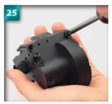
Holding the assembly in your hand, as shown in the photo, insert two 3 × 12mm self-tapping screws into the holes at the top corners. Again, do not fully tighten yet.
