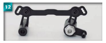
Prepare the steering plate and servo saver assembly built in Stage 26. The steering plate is in the middle, with the two servo savers to the left and right.
