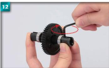
Holding the Allen key so that its shorter arm is in the screw and its longer arm is in your hand will make it easier to tighten, as you are given greater leverage.
