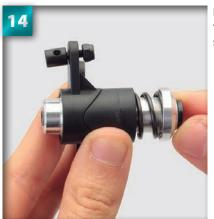
Push the steering post through to the back of the servo saver.
