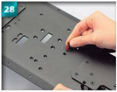
Next locate the holes in the underside of the chassis that lead to the holes of the front torque rod, and insert a  $3 \times 10$ mm countersunk self-tapping screw.
