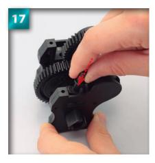
Press the brake cam into place.
