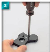
Turn the screw with a screwdriver, making sure the screw enters the gear mount perfectly straight. When you feel the screw reach the far side of the mount, carefully remove the screw, again making sure to keep the screw straight.
