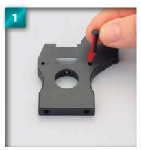
Place the centre gear mount front flat on your work surface, as shown. The centre gear mount front and back parts looks very similar, so make absolutely sure you select the front part. Place one of the 3 × 12mm binding-head screws into the first hole, as shown.
