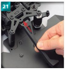
Position the front torque rod beneath the centre of the front upper plate, as shown by the arrow.
