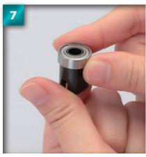
Push the 1680 bearing onto the tip so that it sits flush with the body of the cup joint.
