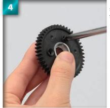
Tighten with a screwdriver, but not too firmly at this stage.
