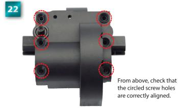
Holding the parts together, insert the first  $3 \times 18$ mm self-tapping screw into the circled hole and tighten lightly.
