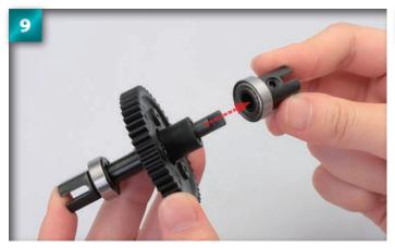
Place the cup joint and bearing assembly onto the tip of the main shaft, as shown. Make sure that the flat portion of the shaft's tip fits into the corresponding flattened section of the inside of the joint (see arrow).
