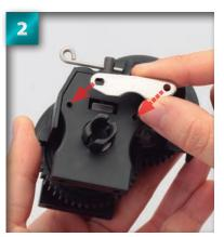
Holding the centre gear mount as shown, place the first brake calliper so that its two holes line up with those on the casing of the mount (arrows). Make sure you have the orientation of the calliper positioned, as shown in the photo.
