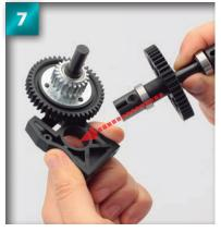
Making sure not to dislodge the main gear, place the centre gear assembly into the second hole on the underside of the gear mount, as shown.
