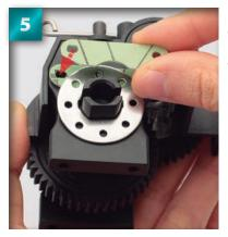
Place the second brake pad over the brake disc, so that its holes line up with those of the first.
