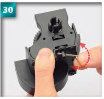
Check that the brake cam is able to rotate by turning the brake cam rod from side to side.
