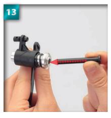
Place one of the steering posts into the hole in the centre of the right servo saver, from the side that houses the spring.
