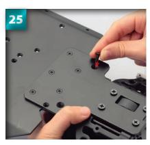
Next, carefully turn the main chassis over, and place a 4 × 10mm countersunk screw into the hole leading to the bottom of the right servo saver.
