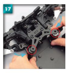
Turn the servo savers until they line up directly with the circled holes on the front upper plate.
