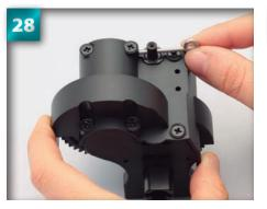
Adjust the rod so that the straight end sits 1mm away from the side of the raised section of the gear case, and the looped end is facing upwards, as shown.
