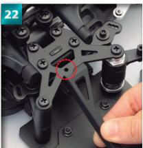
Fit the front torque rod to the upper plate, so that the contours of each are flush with one another.
