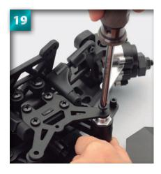
Repeat Steps 18 and 19 for the left servo saver and the second  $4 \times 10$ mm binding-head screw.
