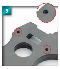
Repeat Steps 1 and 2 for the other hole, so that both holes are left with the screw's indentations, forming the 'tapped' inside (see circles).
