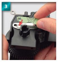
Next, place the corresponding brake pad over the calliper, making sure the holes line up.
