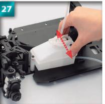
Gently move the tank from side to side. It is OK for it to be able to move a little.
