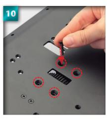
Still holding the centre gear mount carefully in place, tighten the screw with a Phillips screwdriver. Do not tighten fully at this stage.
