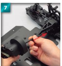
Holding the parts together carefully, fit the other end of the rear driveshaft into the differential cup joint beneath the rear bulkhead.
