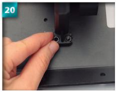
Turn the chassis around and place the second 3mm nut into the next groove in the roll bar.
