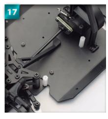
Place the first 3 x 15mm binding-head screw into the hole at the front of the fuel tank.
