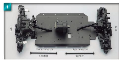
Lay the main chassis assembly (Stage 40) on your work surface facing to the left. Place the centre gear mount (also Stage 40) in the centre, as shown here. Next, lay out both driveshafts – the longer of the two is the rear driveshaft, and the shorter is the front driveshaft. The difference in length is not large, so make sure not to get these confused.
