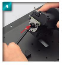
Holding the driveshaft carefully so that the end fitted in Step 2 doesn't fall out of the cup joint, angle the centre gear mount so that its protruding cup joint accommodates the other end of the driveshaft.
