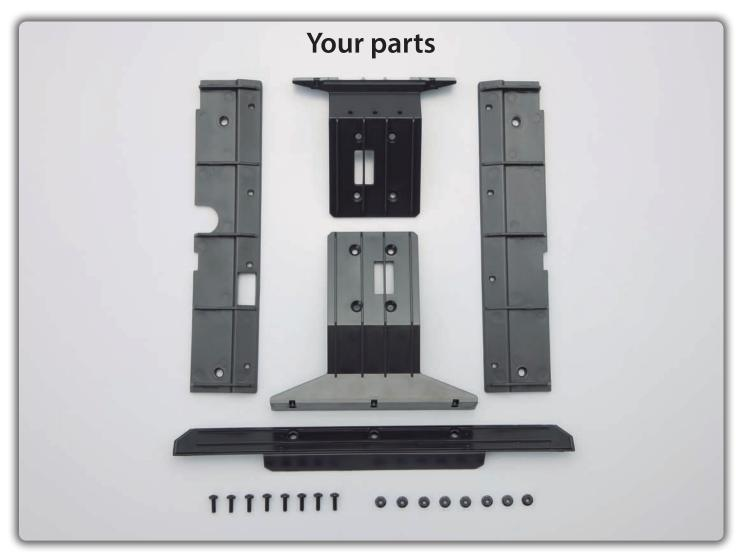
Left body mount base Front bumper mount Rear bumper mount Right body mount base Rear bumper base 3 x 10mm binding-head screws x 8 3mm flange nuts x 8
