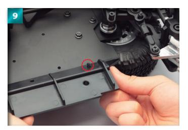
Insert a 3 x 10mm binding-head screw through the first pair of holes from the back.
