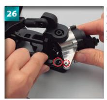
Line up the hole in the front right knuckle arm with that of the free end of the track rod fitted in Step 25.
