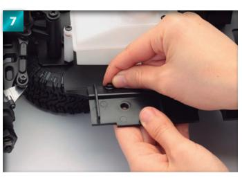
Repeat Steps 4 to 6 for the remaining three pairs of holes to join the left body mount base to the chassis.
