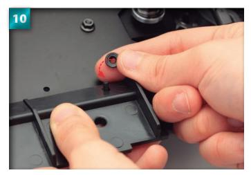
Hold the screw in place and put a 3mm flange nut over the tip of the screw, then tighten by hand.
