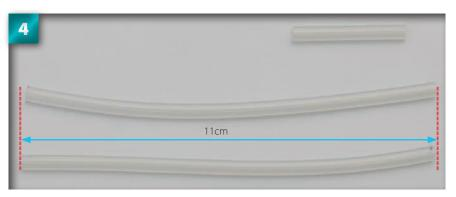
You should be left with two 11cm lengths. Keep the leftover section of tube, as you will be using this at a later stage.
