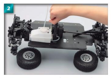
Use the two assembled wheels laid flat on your work surface as a base to raise the main chassis assembly. This will allow you easier access to the side of the chassis.
