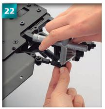
Next, tighten fully using the cross wrench.
