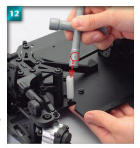
Place the end of the cross wrench marked '8' over the top of the fuel tank post.
