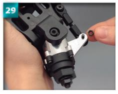
Turn the chassis over and place the second 3mm nut over the tip of the screw.
