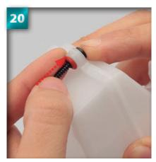
Push the O-ring down so that is rests against the plastic of the tank.
