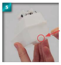
Line up the tip of one of the 11cm lengths of tube to the circled hole in the centre of the tank's bottom edge.
