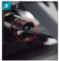
Make sure the metal pin set into the end of the driveshaft fits into the two slots in the cup joint.
