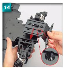
With the holes lined up, begin re-inserting the 4 x 16mm countersunk screws removed in Step 13. Tighten lightly with a screwdriver.
