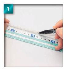
Lay the silicone tube out next to a ruler, perfectly straight. Mark the 11cm point using a pen. Do not stretch the tube.
