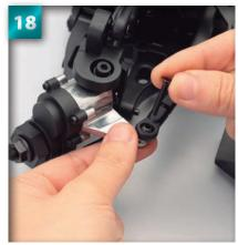
Place a 3 x 18mm countersunk screw through the top of the pillow ball, then through and into the hole in the knuckle arm.
