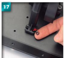
Next, inspect the longer arm of the roll bar – it does not matter if it has come away from the chassis surface a little. Place a 3mm nut into the groove in the tip of the arm, as shown by the arrow.
