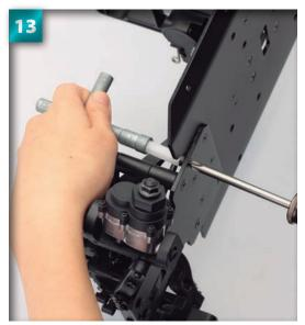
Position the chassis on its side and tighten the screw with a screwdriver, holding the tank post in place with the wrench.
