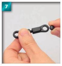
Place a 6.8mm pillow ball into the first of the track rod's sockets. The hole in the ball should be perpendicular to the socket.
