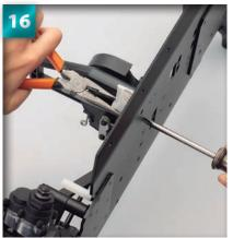
Because of the screw's close proximity to the roll bar, the cross wrench cannot be used for this step. Instead, use the needle-nose pliers – but cover the tank post with some paper towel or tissue first to protect it.
