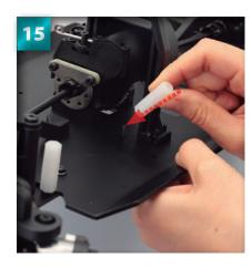
Turn the chassis around again, holding the screw from beneath to prevent it from falling out, then place the second fuel tank post over the tip.
