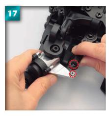
Angle the front left knuckle arm with the free end of the track rod so that the circled holes line up with each other.
