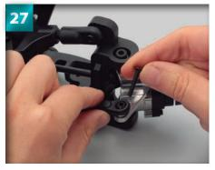
Insert the second 3 x 18mm countersunk screw through the holes in the track rod's pillow ball and the knuckle arm.
