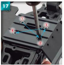
In the order shown in the photo, tighten each screw fully. When the screw stops turning easily, try to perform another half-turn to make sure the part is fastened as tightly as possible.
