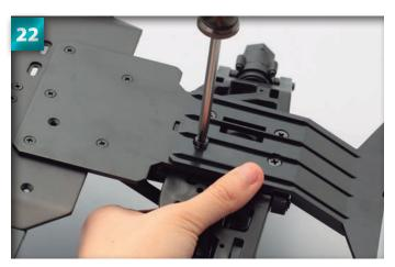
Tighten the remaining three screws lightly.
