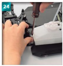
Lightly tighten the first screw using a screwdriver.
