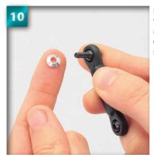
Place a tapered collar over the thin tip of the screw. Make sure the convex side of the collar goes over the screw first.
