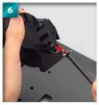
Making sure neither end of the front driveshaft is dislodged, fit the tip of the rear driveshaft into the second cup joint.
