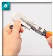
Fold some paper towel or tissue over the part to protect it, then press into place with the needle-nose pliers. Repeat for each socket of both track rods.
