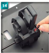
Tighten with a screwdriver, but do not use too much force at this stage – the roll bar should not be rotated by the turning.
