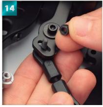
Hold the track rod and countersunk screw in place, and line up a 3mm nylon nut to the tip of the screw.
