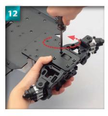
Next, turn the chassis assembly over and begin unscrewing the 4 x 16mm countersunk screws holding the front bulkhead to the chassis.
