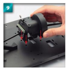
With both driveshafts in place, lower the centre gear mount down onto the surface of the main chassis, so that the four holes line up with those on the chassis.
