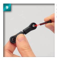
Place a 3 x 18mm countersunk screw through the hole in the pillow ball fitted in Step 8.
