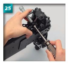
As you did in Step 16, hold the nut in place with the cross wrench and tighten the screw with a screwdriver.
