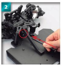
Place one end of the front driveshaft into the differential cup joint facing out of the front bulkhead (circled).
