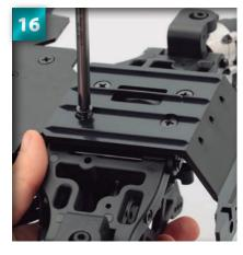
Replace and tighten the remaining three screws. Only tighten these lightly at this stage.
