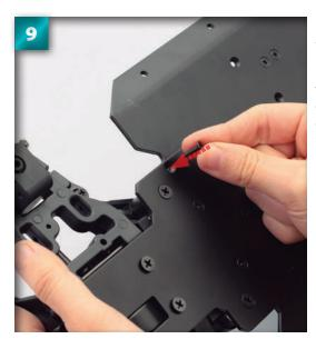
Position the main chassis assembly so that the underside is facing up. Locate the hole shown in the photo at the front end of the chassis, and insert a 3 x 12mm countersunk screw.
