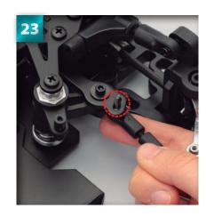
Place the second 3mm nylon nut over the tip of the screw.
