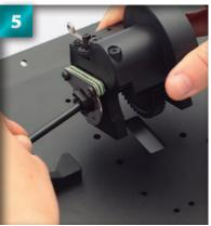
Again, make sure the tip of the driveshaft is fully inserted into the cup joint.
