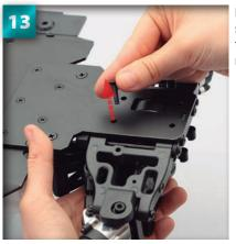
Remove all four screws so that you can remove the bulkhead. Keep the removed screws safely.
