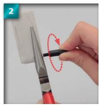
Hold the covered end of the set screw with the needlenose pliers, and screw a 6.8mm ball end over the free end by hand. Turn the ball end until about 8mm of the set screw is inside the part.
