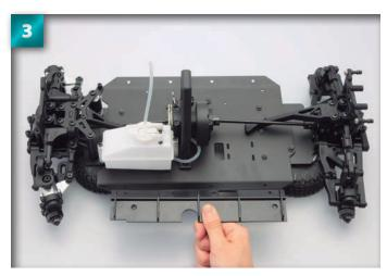
Position the left body mount base next to the left side of the chassis, lining up the row of four screw holes on both parts.
