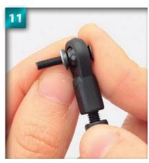
Holding the countersunk screw in place, position the track rod with the tip of the screw facing upwards beneath the hole in the left side of the steering plate (arrowed).
