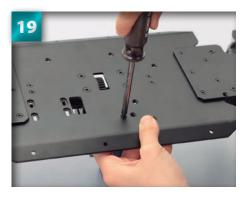
Tighten the screw into the nut with a screwdriver. Be careful not to overscrew, as this can damage the inside of the nut.
