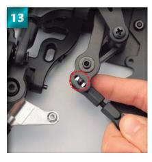
Push the tip of the screw through the central hole in the steering plate (circled).
