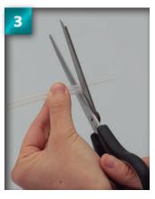
Using scissors, cut the remainder of the silicone tube to the same length.
