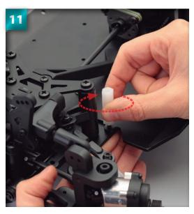
Holding the screw in place from beneath, turn the fuel tank post clockwise to fasten the part.
