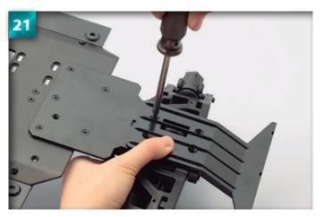
Begin re-inserting and tightening the screws removed in Step 19. Only tighten these lightly at first.
