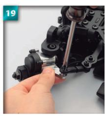
Carefully turn the chassis over and place a 3mm nut onto the tip of the screw.
