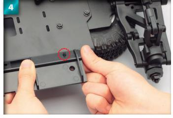
Insert a 3  $\times$  10mm binding-head screw through the first pair of holes from the back.
