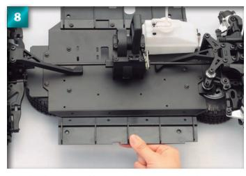
Turn the chassis assembly around and position the right body mount to the right side of the chassis, as you did for the left.
