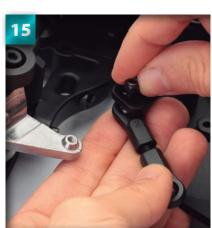
Position the chassis on its side and hold the nut in place with the end of the cross wrench marked '5.5'. Place the Phillips screwdriver into the head of the countersunk screw.
