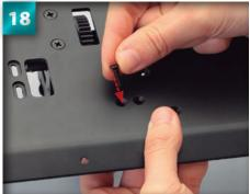
Holding the nut in place with your finger, turn the chassis around and place a 3 x 12mm countersunk screw into the corresponding hole on the underside of the roll bar.
