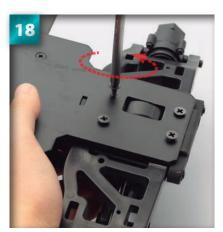
Remove all four screws so that you can remove the rear bulkhead.
