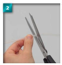
With scissors or a knife, cut the tube at the 11cm mark. If you use a knife, be sure to place the tube on a cutting mat.
