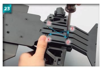
In the order shown in the photo, tighten each screw fully. When the screw stops turning easily, try to perform another half-turn to make sure the part is fastened as tightly as possible.
