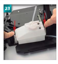
Press down on the screws until you feel them slot into the holes in the tank posts.
