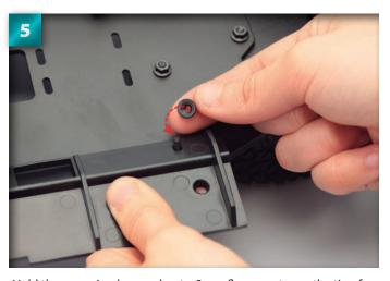
Hold the screw in place and put a 3mm flange nut over the tip of the screw.
