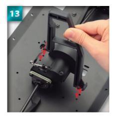
Turn the chassis assembly around, then place the roll bar over the centre gear mount, as shown. The shorter arm will sit on the centre gear mount itself, and the longer on the surface of the chassis (see arrows).
