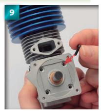
Place one of the  $2.5\times8$ mm cap screws into the topright hole.
