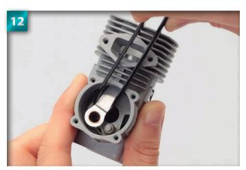
Use tweezers, or needle-nose pliers wrapped in tissue, to lift the connecting rod over and on top of the pin of the crankshaft.
