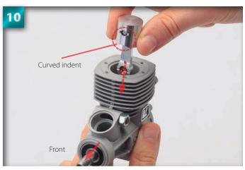
Slowly slide the piston, connecting rod side first, into the top of the crankcase. Make sure the bottom edge of the piston that has a shallow, curved indent in it faces the front of the crankcase.
