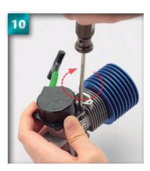
Tighten the remaining screws into place. Do not overtighten, as the black plastic of the recoil starter case is soft and may warp under too much pressure.
