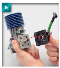
Carefully press the parts together.
