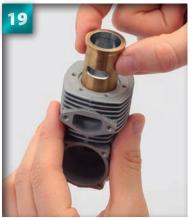
Once aligned, gently slide over the piston so that the cylinder enters the crankcase.
