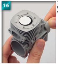
The piston should be sitting flush with the top edge of the crankcase chamber.
