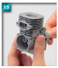
Now slowly rotate the crankshaft so that the pin is at the top of the crankcase, with the counterweight at the bottom.
