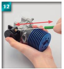
You can now test the recoil cord. Do not pull too hard, though. It should be pulled back into the case when released.
