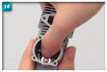
Once the parts are fitting together comfortably, press the rod completely onto the pin using your thumb.
