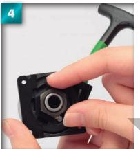
Press the bearing into place so that it fits neatly.
