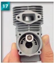
With the back side of the crankcase and the rear scavenging port both facing you, line up the cylinder with the raised piston.
