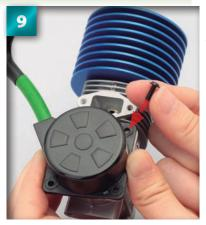
Place the first of the  $2.5 \times 8$ mm flange screws into the top right hole.
