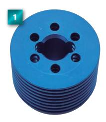
Familiarise yourself with the cylinder head. The large hole in the top will accommodate the glowstarter plug, and the six smaller holes will be used for screws to attach the part to the crankcase.
