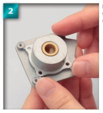
Line up the gasket so that the four holes line up with those on the rear plate.
