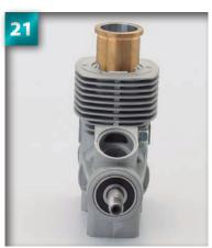
Turning the cylinder gently from side to side, continue to lower the part into the crankcase. Make sure that the piston remains in its current position.
