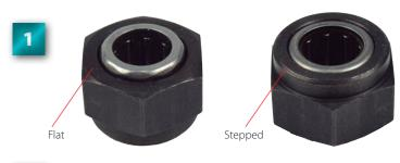
Inspect the one-way bearing. The bearing can be rotated one way but not the other, so it is very important it is fitted correctly. Make a note of the flat and stepped sides, shown in the photo.
