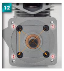
Once all four cap screws are in lightly, tighten each fully following the diagonal pattern shown in the photo.
