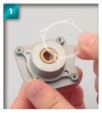
Fit the gasket over the central raised section of the rear plate. It does not matter which way round the gasket goes.
