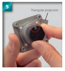
Hold the rear plate as shown, with the triangular projection to the right. Rotate the back of the recoil starter shaft until the notch (circled) is facing the top edge.
