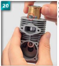
Lower the cylinder into the crankcase, stopping to check the alignment of the rear port is at the point circled.
