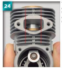
This photo shows how your assembly should look, with the scavenging port fully aligned with the exhaust port (see dotted red lines).
