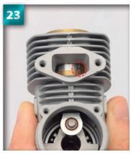
Make sure that the rear scavenging port at the back of the assembly is in line with the exhaust port of the crankcase. The photo shows the incorrect positioning of the parts – note the misaligned edge of the rear scavenging port (circled).
