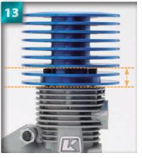
Tighten each screw lightly until they are sitting inside their respective holes, protruding up to about the third fin.
