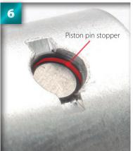
Take a close look at the piston itself. It is connected to the rod by the piston pin, which is in turn prevented from falling out by the piston pin stopper (highlighted).
