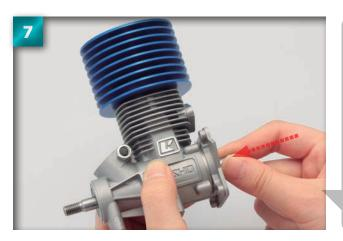
If the gasket gets dislodged as you join the parts, adjust it carefully with tweezers. It should sit perfectly level with the edge of the crankcase (see
