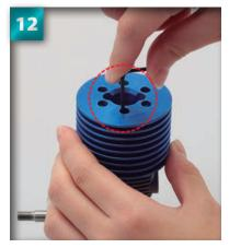
Guide the cap screws down through the fins until they rest four fins up from the bottom (orange arrows).
