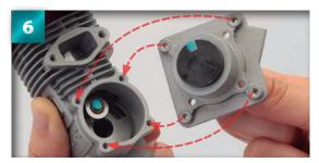
Holding the shaft in place, line up the rear plate to the back opening of the crankcase. The red arrows show how the screw holes will line up, and the blue dots show how the notch will accommodate the piston's connecting pin.
