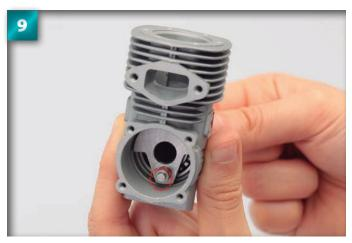
Holding the crankcase assembly as shown, rotate the crankshaft so that its connecting pin (circled) is at the bottom of the crankcase, known as 'bottom dead centre'.
