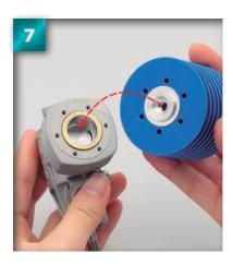
Making sure the gaskets do not fall off, join the parts as shown in the photo.
