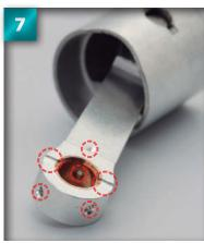
Looking down into the piston shows the connecting rod, piston pin and stopper (circled).
