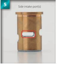
There are two smaller ports on either side. These will support the front intake port.
