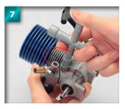
Turn the cross wrench until the nut tightens enough so that the wrench stops turning freely, then stop so as not to overtighten it.
