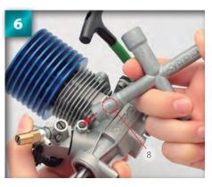
Using the hole marked '8' on the cross wrench, fit over the carburettor nut.
