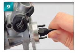
Tighten the pilot shaft as far as you can by hand only.
