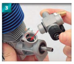
Holding the crankcase assembly in one hand, lower the carburettor into the carburettor mount of the crankcase. Make sure the fixed carburetor shaft (circled) that will hold the part in place is positioned so that its curved indent is matching the inside corner of the mount. This way the carburetor will fit snugly into the mount.
