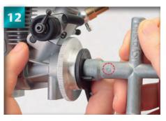
Keep holding the flywheel in place, and put the arm of the cross wrench marked '10' over the pilot shaft.
