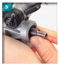
Push the collet along the shaft. The collet should rest against the bearing. It does not matter where the split in the collet is situated.
