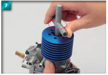
Once the glow plug is in perfectly straight, tighten it into place by turning the wrench.
