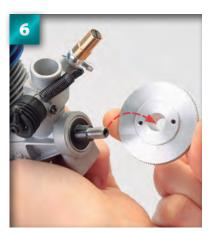
Next, place the flywheel, flat side first, over the shaft and collet so that it will fit as it did in Step 3.
