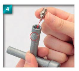
Carefully place the top of the glow plug into the hole marked '8' on the cross wrench.
