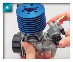
Gently push the carburettor into the mount. Twist it from side to side gently to help it in if it is stiff.
