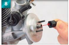
Line up the threaded portion of the pilot shaft with the tip of the crankshaft.
