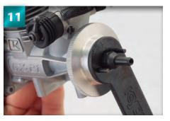
Press the flywheel wrench firmly against the surface of the flywheel. It is important that there is no gap between the wrench and the surface, as this may lead to the pins being bent.
