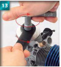
To secure the parts, turn the flywheel wrench anticlockwise and the cross wrench clockwise. This will push the flywheel further over the tapered collet so that it'bites' and fastens to the pilot shaft.
