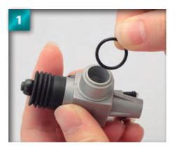
Place the O-ring over the cylindrical projection of the carburettor.
