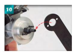
Line up the flywheel wrench with the pilot shaft and the pins in the flywheel.
