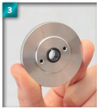
Slide the wide rim (bottom) of the tapered collet over the tip of the crankshaft.
