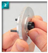
Place the tapered collet, narrow side first, into the hole in the centre of the flywheel, from the side that does not have pins in it.
