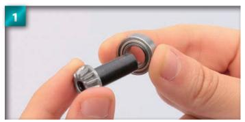
Hold the pre-assembled driveshaft and place the bearing 1680 onto the shaft so that it rests behind the gear.
