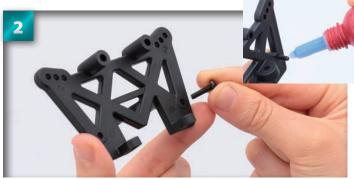
Insert a 3  $\times$  12mm screw into the hole on the rear of the damper stay and apply some lock agent to the thread (inset).
