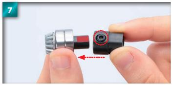
Slide the cup joint onto the end of the shaft, positioning it so the set screw is placed over the flat section of the shaft (red rectangle).
