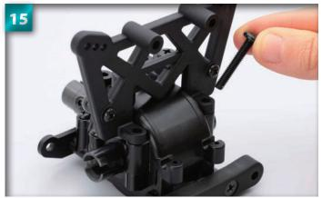
Insert one of the  $4\times25$ mm screws into the hole on the lower projection on the rear of the stay.
