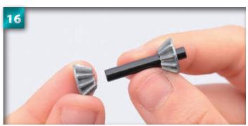
Slide a 10T bevel gear onto each end of the bevel gear shaft,
