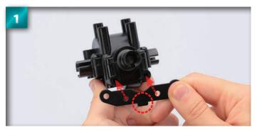
Holding the assembly from the previous stage as shown, position the rear lower suspension plate below the driveshaft. The red circle should help you identify the position of the plate.
