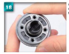
Align the four screw holes of the gear with those of the case.
