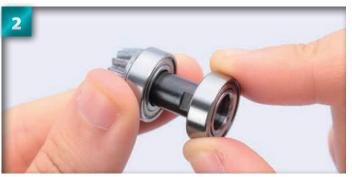
Place the second bearing onto the driveshaft, up against the first.
