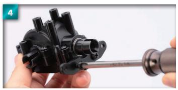
Tighten another 4 x 10mm screw into the suspension plate hole to the left of the one in the previous step.
