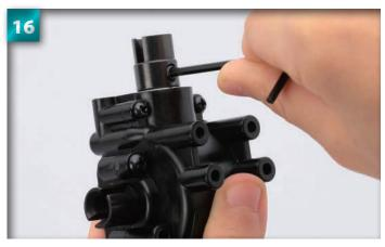
If the fit is too tight, loosen the set screw with the Allen key.
