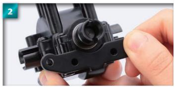
Align the screw holes of the rear lower suspension plate with those of the bulkhead.
