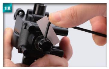
Use the Allen key to tighten the set screw again, to secure the joint in place, and then remove the wedge.
