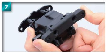
Align the screw holes of the lower suspension holder with those of the bulkhead.
