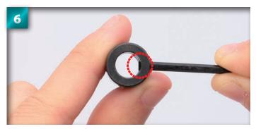
Keep tightening the set screw into the hole until about 0.5mm of the tip is visible from the inside of the cup joint.
