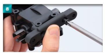
Insert one of the  $4\times16$ mm countersunk screws into one of the holes of the holder and tighten it to the bulkhead.
