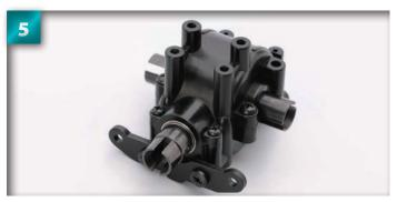
This is how the assembly should look now, with the rear lower suspension plate attached.
