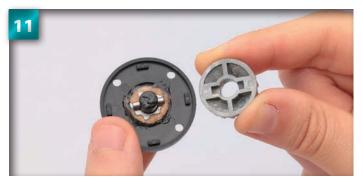
Hold the 20T bevel gear, as shown. Locate the groove on the back of the gear.
