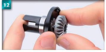
Align the groove on the back of the bevel gear with the position of the pin and place the gear into the back of the case, sliding it over the joint.
