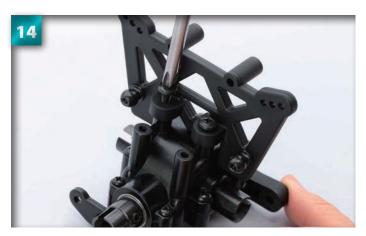
Repeat this process, tightening a  $4 \times 10 \text{mm}$  screw into the hole on the other side.
