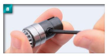
Tighten the set screw slightly, just enough to stop the cup joint moving around the shaft.
