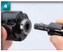
Place the 6mm O-ring over the joint on the inside of the case.
