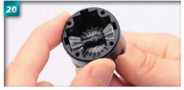
Hold the differential case and slowly turn the joint to spread the grease over the gears.
