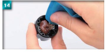
Apply a large amount of grease into the back of the differential case.
