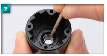
Apply some grease to the recess in the centre of the inside of the differential case.
