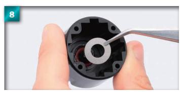
Place the  $6 \times 12$ mm shim over the joint and push down to rest on the O-ring.
