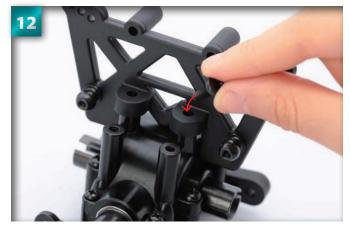
Insert one of the  $4 \times 10$ mm screws into one of the holes in the semicircular projections on the front side of the damper.
