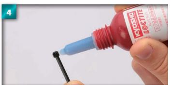
Insert the tip of the Allen key into the hexagonal hole in the 5  $\times$  4mm set screw and apply a small amount of lock agent to the thread of the screw.
