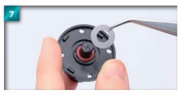
Place the  $6 \times 12$ mm shim over the joint and push it down to rest on the O-ring.
