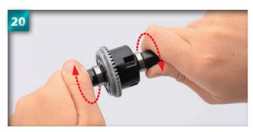
Turn the cup joints in opposite directions to spread the grease around the internal gears.
