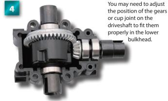
Slowly turn the driveshaft clockwise to check that the differential gear rotates smoothly. When doing so, make sure that the parts remain in their correct positions in the bulkhead.
