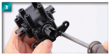
Insert a  $4 \times 10$ mm screw into the hole on the right of the suspension plate and tighten into place.
