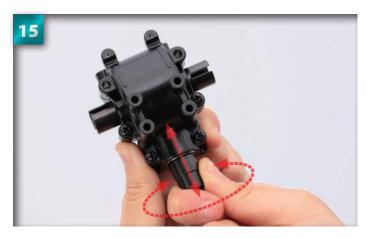
Once the upper bulkhead is secured, test the driveshaft. Turn it from left to right while moving it back and forth slightly to find the best position for it, where the gears and joints of the assembly rotate smoothly.
