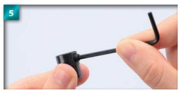
Insert the set screw into the hole in the side of the cup joint.
