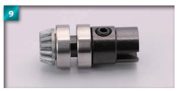
Keep the driveshaft assembly close to hand as it will be used a few steps further on.
