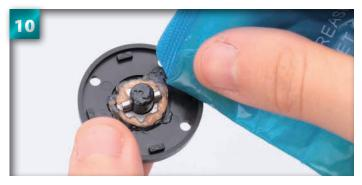
Smear some extra grease around the shim and the joint.
