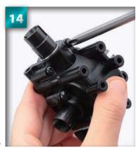
Tighten the first 3 x 10mm screw into the hole.
