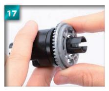
Place the 43T gear over the end of the joint.
