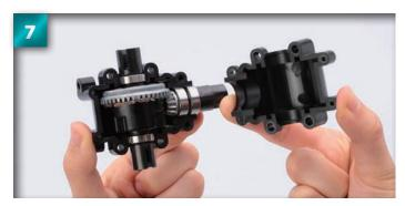
Place the upper bulkhead over the differential and shaft, aligning it with the lower bulkhead.
