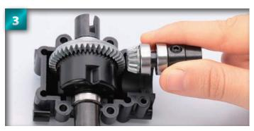
Place the driveshaft in the cylindrical recess to the side of the differential in the lower bulkhead.
