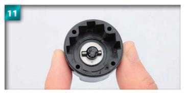
Adjust the position of the pin so that it protrudes evenly from both sides of the joint.
