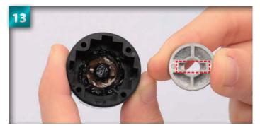
Hold the 20T bevel gear as shown. Locate the highlighted groove on the back of the gear.
