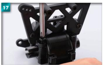
Fit the second 4 x 25mm screw into the hole in the projection on the other side and tighten it, securing the stay to the bulkhead.
