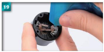
Squeeze a generous amount of grease into the back of the differential case.
