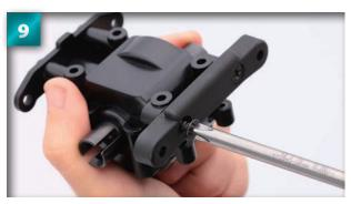
Tighten a  $4 \times 16 \text{mm}$  screw into the second hole of the suspension holder.
