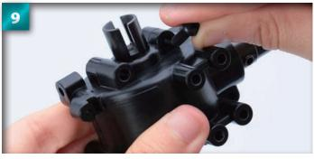
Place one of the  $4 \times 12$ mm screws into the hole to the right of the joint shaft.
