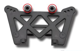
Identify the rear damper stay. The two posts (circled) project in only one direction, to the rear.
