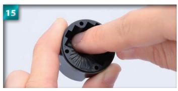
Push the bevel gear down onto the joint until the pin slots into the groove.
