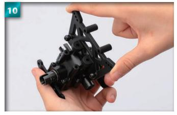
Align the holes of the semicircular projections on the front of the damper stay with those of the two projections on the bulkhead.
