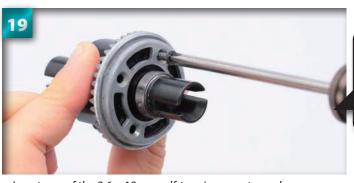
Insert one of the  $2.6 \times 12$ mm self-tapping countersunk screws into one of the holes and tighten until halfway in. Then, following the order shown in the diagram on the right, tighten the next three screws halfway into their holes, and when all four are in place, fully tighten them in the same order.
