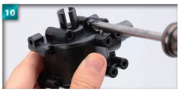
Tighten the screw into the hole, keeping it as straight as possible.
