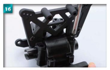
Tighten the 4 x 25mm screw into the hole.
