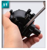
Place the second 4 x 12mm screw into the hole on the opposite side of the assembly, next to the other joint shaft of the differential.
