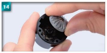
Align the groove on the back of the bevel gear with the position of the pin and insert the gear into the back of the case, sliding it over the joint and the pin.
