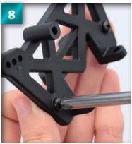
Tighten the screw completely into the flange ball with a Phillips screwdriver.
