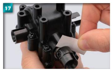
Wedge a piece of thin card or similar between the joint and bearing to hold the cup at the correct distance.
