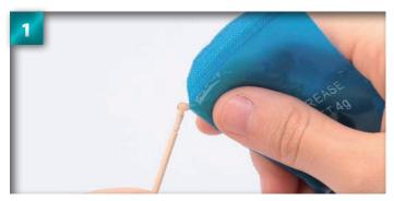
Cut a corner from the grease bag and place a small amount of grease onto the end of a toothpick, or similar.
