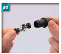
Temporarily assemble the shock by inserting the shaft assembly into the shock case.
