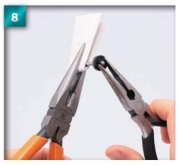
When you can no longer turn the nut by hand, use pliers to turn it by one more revolution.
