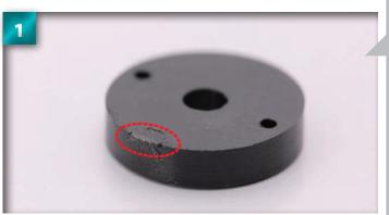
Check the parts for any burrs and scrape off any that you find with a cutting knife, following the advice shown on the right.
