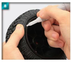
When the glue is dry, turn the wheel assembly over and repeat Step 7 for the other side.
