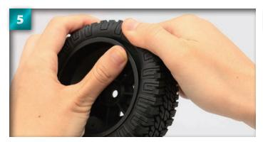
Working around the wheel, pull the shoulder of the tyre back slightly to help ease it into the groove on the inside of the rim.
