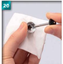
Take the shock shaft assembly and insert it into the hole in the centre of the shock cap.
