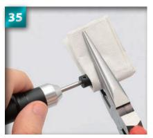
Place folded tissue paper around the ball end and press into place with pliers.
