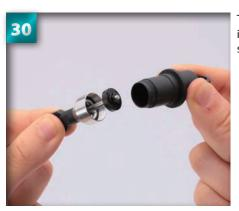
Temporarily assemble the shock by inserting the shaft assembly into the shock case.
