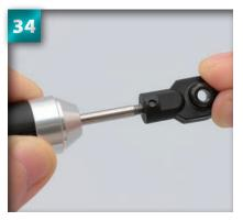
Push the pillow ball into the hole in the ball end, keeping the hole in the ball aligned with that of the ball end.
