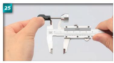
Measure the gap between the cap and the ball end. The ball end should be positioned 14mm away from the cap, so adjust the fit if necessary by either tightening or loosening it.
