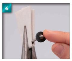
Place the second 2.3mm washer onto the end of the shaft, sandwiching the piston.
