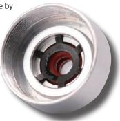
Holding the cap with tissue paper, pour a few drops of shock oil over the O-rings and stopper ring.
