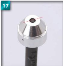
Push down hard on the shock cap until the tip of the rod is flush with the cap. The stopper ring's angled projections (see Step 9) should slot into the ridge on the inside of the shock cap, so that the two O-rings remain inside when the rod is removed (see photo in Step 18).
