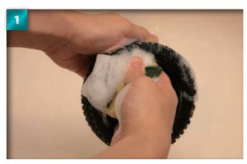
Wash the tyre with some washing-up liquid, paying especially close attention to the areas that will be in contact with the wheel rims.
