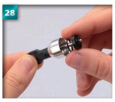
Once the piston is through the 11mm O-ring, drop the ring down inside the shock cap.
