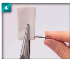
Place the 2.3mm washer over the exposed end of the shaft.
