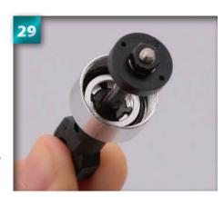
The O-ring should rest in the groove on the inside of the shock cap, as shown.
