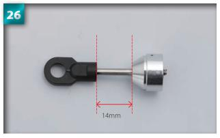
The gap between the cap and the ball end must be 14mm. If you don't have any callipers to measure it, just use a ruler.
