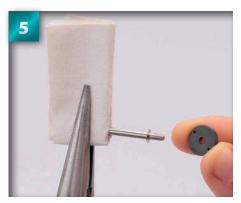
Place the piston onto the end of the shaft, up against the washer.
