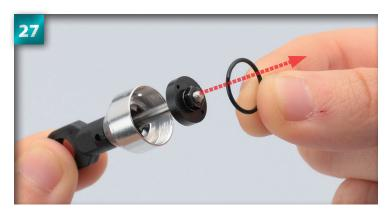
Push the shaft through the cap and then pass the piston through the 11mm O-ring.
