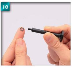
Place the stopper ring onto the end of the shock assembly rod.
