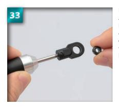
Hold the shock assembly so that the larger side of the ball end is uppermost. The 6.8mm pillow ball will fit into the hole in the ball end.
