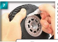
Ease the sidewall back a little, creating a small gap between the tyre and the wheel rim, then squeeze a small amount of instant adhesive into the gap. See the Tip box below for the recommended technique for applying the glue.
