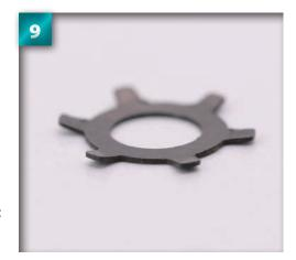
Place the stopper ring on a flat surface, with the projections around the sides angled up.
