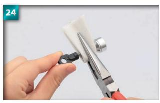
Screw the ball end onto the shaft until you can no longer see the thread of the shaft.
