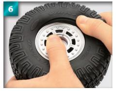
Turn the wheel assembly over and position the other side of the tyre into the groove on the other side of the wheel.
