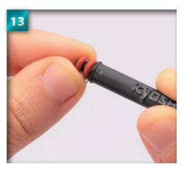
Slide the second O-ring onto the rod up against the first.
