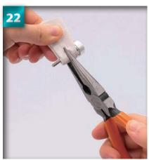
Insert the shaft into the hole on the 6.8mm ball end.
