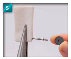
Place the shock piston onto the end of the shaft, up against the washer.
