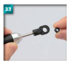
Hold the shock assembly so that the larger side of the ball end is uppermost. The 6.8mm pillow ball will fit into the hole in the ball end.
