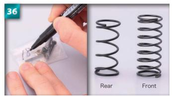
Store the unused parts safely in a plastic bag, marking the stage number for reference. Also, note the difference between the front and rear shock springs: the front has a greater number of coils than the rear, giving it a higher 'pitch'.
