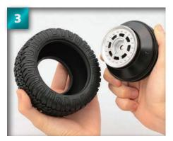
Hold the tyre and wheel as shown. The wheel must enter the tyre through the wider hole.
