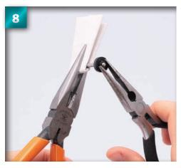
When you can no longer turn the nut by hand, use pliers to turn it by one more revolution.
