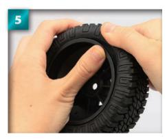
Working around the wheel, pull the shoulder of the tyre back slightly to help ease it into the groove on the inside of the rim.
