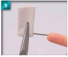
Hold the end of the shock shaft wrapped in tissue paper with pliers. Pick up one of the 2.3mm washers.
