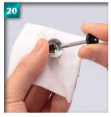
Take the shock shaft assembly and insert it into the hole in the centre of the shock cap.
