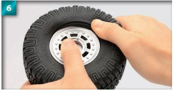
Turn the wheel assembly over and position the other side of the tyre into the groove on the other side of the wheel.
