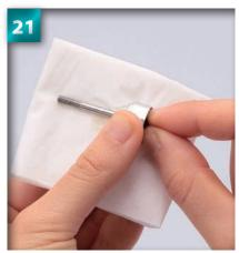
Push the shaft all the way into the cap. Wipe off any oil from the shaft.
