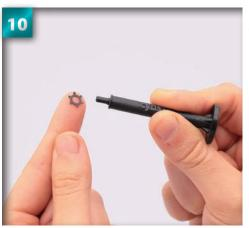
Place the stopper ring onto the end of the shock assembly rod.
