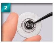
Make sure the two depressions on the hub cap (circled) are aligned horizontally with the lettering 'CTIS' on the sticker.
