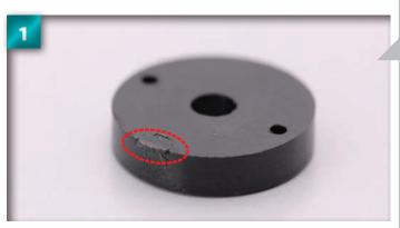
Check the parts for any burrs and scrape off any that you find with a cutting knife, following the advice shown on the right.
