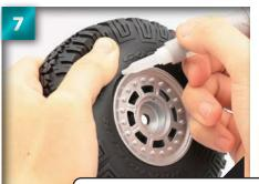
Ease the sidewall back a little, creating a small gap between the tyre and the wheel rim, then squeeze a small amount of instant adhesive into the gap. See the Tip box below for the recommended technique for applying the glue.
