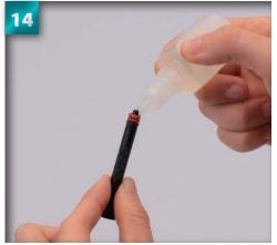
Apply a small amount of shock oil to the O-ring at the end of the rod.
