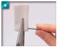
Place the 2.3mm washer over the exposed end of the shaft.
