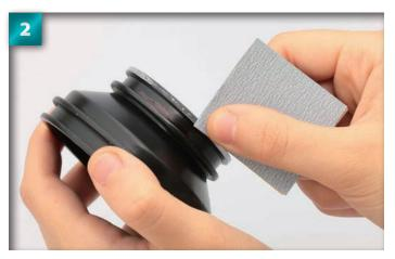
While waiting for the tyre to dry, use wet and dry paper to remove the paint from the wheel rims provided in Stage 1. This will help with adhesion.
