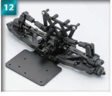
From the front, your assembly should look like this. Note the positioning of the holes on the plate.
