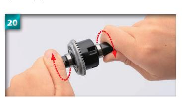
Turn the cup joints in opposite directions to spread the grease around the internal gears.
