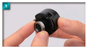
Place the 1510 ball bearing onto the cylindrical segment of the differential case, making sure it is on straight.
