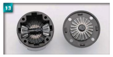
Push the bevel gear down onto the joint until the pin slots into the groove. Retrieve the differential gear assembly from the previous stage.
