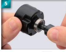
Turn the joint from right to left to spread the grease. If grease builds up between the ball bearing and the case, wipe it with tissue paper.
