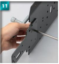
Hold the crosswrench over the flange nut to stop it from moving, and begin to tighten the screws from the other side, this time using a screwdriver. Turn until the hold is firm, and repeat for all five sets of screws and flange nuts.
