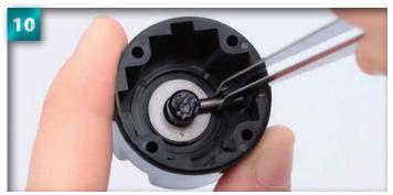
Carefully insert the metal pin through the hole with the tweezers, as shown. Using the recesses cut into the inside of the differential case will allow you more space to position the pin.
