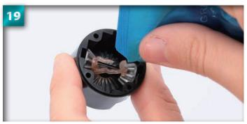
Liberally apply grease to the inside of the differential case, but do not finish the bag of grease, as you will need it in future stages.
