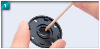
Place a small amount of grease onto the end of a toothpick, and apply some grease to the recess in the centre of the inside of the differential case.
