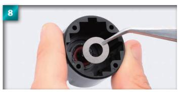
Next, place the 6 x 12mm shim over the shaft so that it rests at the base, covering the O-ring. It does not matter which way round the shim goes.
