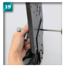
As you did in Stage 11, firmly tighten each set of screws and flange nuts by using the crosswrench and Phillips screwdriver.
