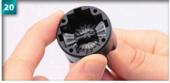
Holding the differential case steady, slowly turn the joint from the back to distribute the grease evenly among the moving parts.
