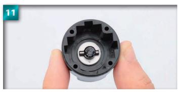
Your assembly should look like this, with equal parts of the metal pin visible on each side of the joint.
