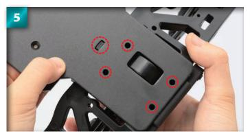
Turn the parts over, holding them together carefully to prevent the assembly slipping. Check that the holes are properly aligned.
