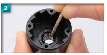
Using the toothpick, spread the grease around the groove on the inside of the differential case, as shown. Use just enough so that the groove shines slightly.
