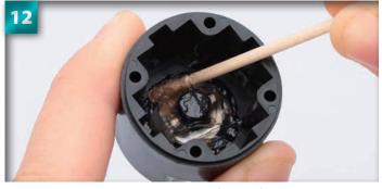
Liberally apply grease to the inside of the differential case, covering the shim and joint.
