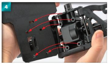
Hold the rear chassis plate with the front facing upwards in one hand, and with the other line up the rear bulkhead you assembled in Stage 16. Line up the holes shown by the arrows.
