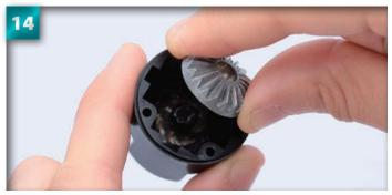
Slide the bevel over the tip of the joint so that the groove on the back lines up with the metal pin.
