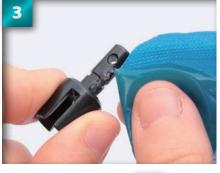
Now apply some grease to the thin end of the differential cup joint. Use the photo to gauge a suitable amount.
