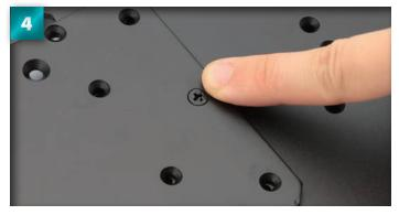
The screw will go right through both holes so that its countersunk head sits flush with the plate's surface. At this stage, the screw is still moving freely within the hole.
