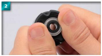
Using both thumbs, push down on the ball bearing evenly, being careful not to apply too much pressure, as this could damage the ball bearing.
