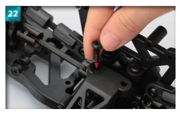
Insert one of the  $4 \times 10$ mm binding-head screws into the hole on the torque rod (see arrow).
