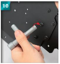
Line up the side of the crosswrench supplied with Stage 8 marked '5.5' with one of the flange nuts, as arrowed.
