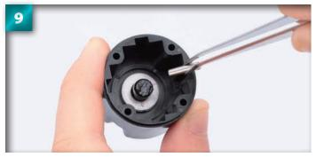
Using tweezers, carefully line up the  $2.5 \times 10.3$ mm metal pin with the hole drilled through the differential joint.
