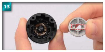
Make a note of the rectangular groove in the back of the 20T differential bevel. The metal pin you fitted in Stage 10 will sit inside this once fitted.
