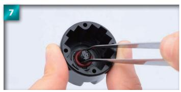
Part the tweezers slighty, and gently push the O-ring down into the groove at the base of the joint.
