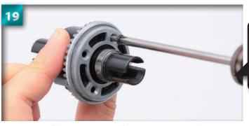
Insert one of the  $2.6\times12$ mm self-tapping countersunk screws into one of the holes and tighten until halfway in. Then, following the order shown in the diagram on the right, tighten the next three screws halfway into their holes, and when all four are in place, fully tighten them in the same order.
