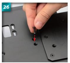
Insert a 3  $\times$  10mm countersunk screw into one of the holes, making sure it is lined up with one of the holes on the end of the torque rod behind.
