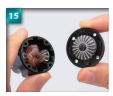
Locate the four screw holes on both the differential case and cap assemblies.
