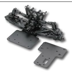
This stage is complete. Store the parts away safely, resting both chassis plates flat during storage to lower the risk of their becoming bent out of shape.
