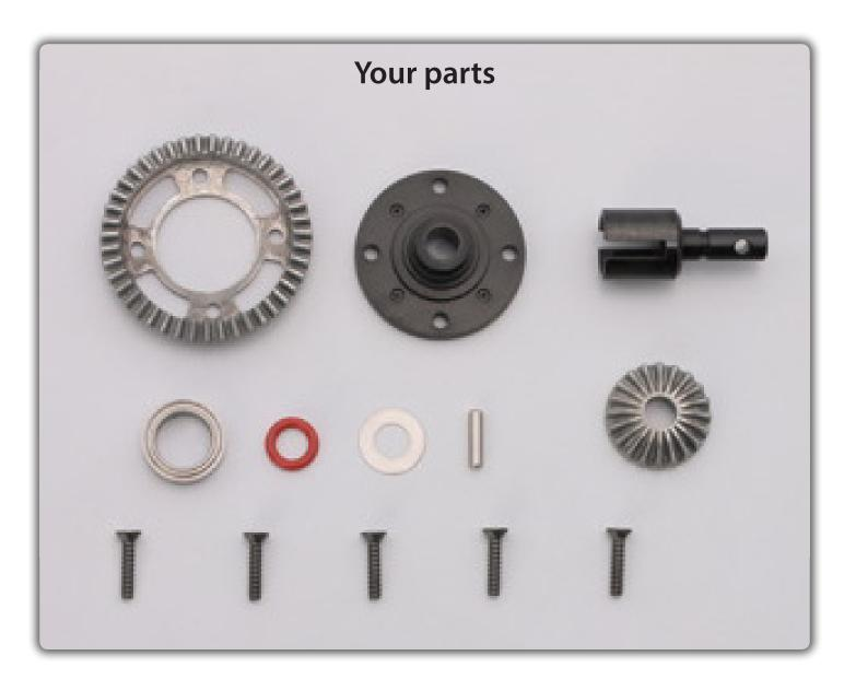
Differential ring gear (43T) Differential cap Differential cup joint 1510 ball bearing 6mm O-ring 6 × 12mm shim 2.5 × 10.3mm metal pin Bevel gear (20T) 2.6 × 12mm countersunk screws x 5
