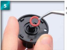
Place the 6mm O-ring over the end of the joint.
