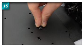
Rotate the chassis and tighten a flange nut by hand onto the tip of the screw, as you did in Stage 6.
