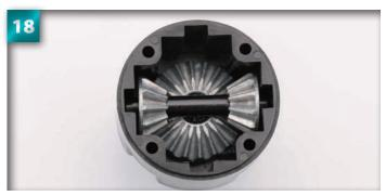
Once in place, slide the two 10T bevels apart as far as they will go. At this point, they should slot neatly into place with the teeth of the 20T bevel beneath.
