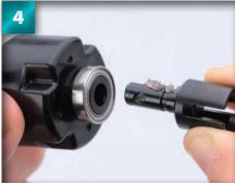
Turn the differential case around, and using tweezers, place the 6mm O-ring over the tip of the joint inside.
