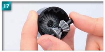
With the 10T bevels together as shown in the photo, place the bevel shaft into the differential case. The ends of the bevel shaft should fit into the recesses in the side of the case.
