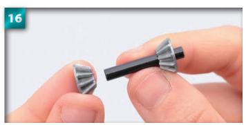
Slide each of the 10T bevels onto the bevel shaft, so that they are facing each other.
