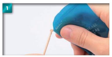
Apply a little of the grease you kept from Stage 11 to the tip of a toothpick.
