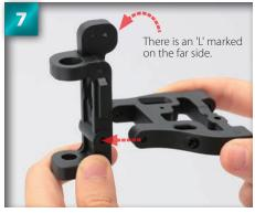
Holding the left hub carrier as shown, line up the left suspension arm - the holes on the narrow end of the suspension arm should sandwich those on the body of the hub carrier (see arrows). The side of arm marked 'L' should be facing upwards, closest to you.
