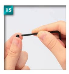
Apply a little threadlocking adhesive to the threaded portion of the set screw. Rubber-based adhesive can also be used.
