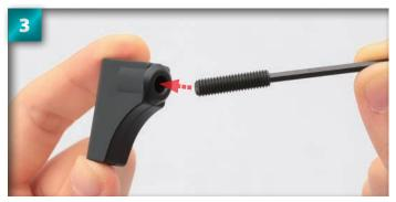
Place the tip of the shaft into the corresponding hole on one of the front upper arms, making sure to enter the hole perfectly straight to avoid damaging the threads.
