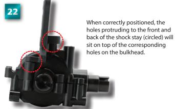
Insert a 4 x 25mm bindinghead screw into one of the holes on the front of the shock stay.
