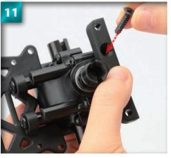
Insert a 4 x 16mm countersunk screw through one of the holes in the holder and into the bulkhead. Make sure the holder is positioned the right way round, with the contoured section fitting to the curve of the cup joint.
