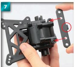
Line up the front lower suspension plate with the holes on the front side of the bulkhead (see arrows). Make sure the circled projection on the plate is positioned as it is in the photo.
