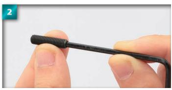
Make sure the shaft is fitted onto the longer arm of the Allen
