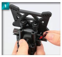
Place a 4 x 12mm round-head screw into the hole on the back right side of the front bulkhead (see arrow).
