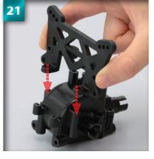
Position the front shock stay onto the top of the upper bulkhead, checking against the photo that you have placed it the right way round.
