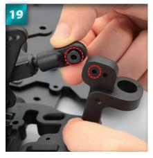
Line up the upper suspension arm's ball end and flange ball with the left front hub carrier you fitted in Stage 27. Make sure the hole in the flange ball is positioned against the circled hole on the hub carrier.
