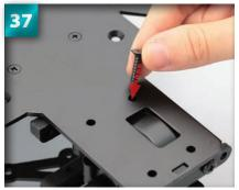
Insert a 4 x 16mm countersunk screw into one of the holes.
