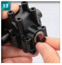
Turn the protruding end of the driveshaft so that the flat (D-cut) section is facing upwards (see red shading).
