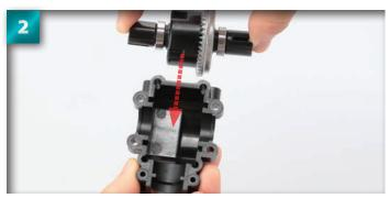
Place the differential you assembled in Stage 24 carefully into the lower bulkhead, with the ring gear on the right side of the bulkhead.
