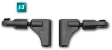
Repeat Steps 1 to 12 to build the second upper suspension arm. The two assemblies should look like this – make sure the 3mm gap between the sections of the arms are matching.
