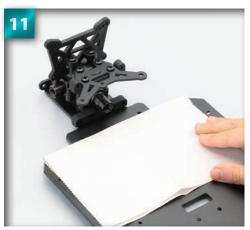
Lay the chassis and bulkhead assembly you built in Stage 26 on your work surface, with the back end of the front bulkhead facing you. Lay some tissue paper over the chassis plates.
