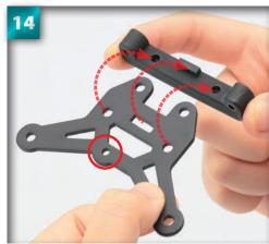
Line up the front bulkhead plate with the front suspension holder, following the red arrows. Make sure the hole in the middle portion of the bulkhead plate (circled) is slightly to the left of centre.
