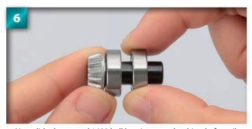
Now slide the second 1680 ball bearing over the driveshaft until it rests in the middle, leaving a space between it and the first.
