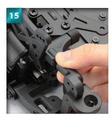
Position the upper suspension arm as shown, so that the holes in the front and back of the part line up with those on the shock stay and bulkhead.
