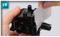
Slot a single piece of paper in between the cup joint and the bulkhead. If the paper gets stuck, tease the cup joint back a fraction. This is to establish the correct gap between the two parts.
