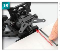
Repeat Step 13 for the right side of the bulkhead, again making sure not to push the suspension shaft too far at first.
