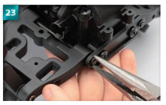
Clip an E-ring over the tip of the shaft as you did in Step 18 to complete the assembly of the front lower suspension arms.
