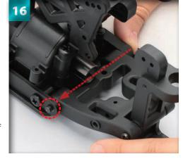
When placed correctly, the tip of the suspension shaft should be visible on the far side, as shown.
