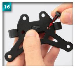
Place a 4 x 10mm binding-head screw into one of the holes of the bulkhead plate.
