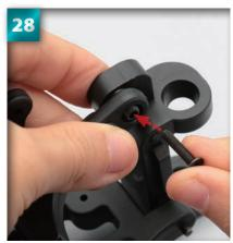
Hold the parts together and insert a 3 x 15mm countersunk screw into the hole in the ball-shaped side of the flange ball (arrowed).
