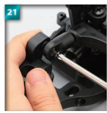
Check that the suspension arm is able to move back and forth slightly.
