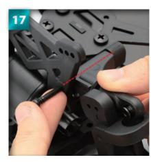
Once the shaft has entered every hole, tighten with a screwdriver. Stop as soon as the head of the screw rests against the shock stay.
