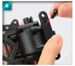
Insert a 4 x 10mm binding-head screw through one of the holes on the plate and into the hole on the bulkhead.
