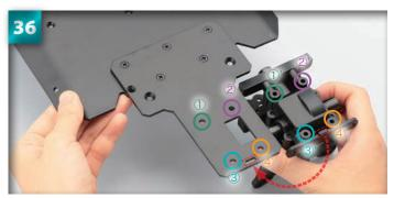
Position the chassis with the underside facing you. With the front bulkhead assembly also underside-up, align the holes, using the numbers and arrows in the photograph as a guide.
