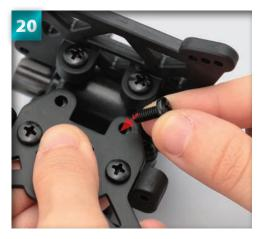
Insert a 4 x 10mm binding-head screw into one of the holes on the plate.
