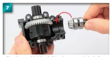
Place the assembled driveshaft into the recess at the back of the lower bulkhead (arrowed).
