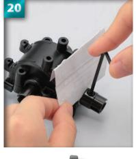
Now tighten the set screw with the Allen key. The paper should be able to come out without tearing.
