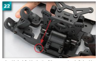
As with the left side, the tip of the suspension shaft should be visible.
