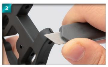
Use a knife to carefully remove any burrs.
