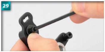
Tighten with the 2.5mm Allen key. Once fully tightened, loosen by one half-turn.
