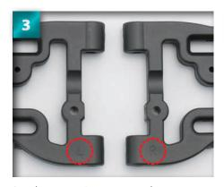
Lay the suspension arms together on your work surface - you will see that they are marked L and R for left and right.
