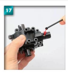
First make sure that the flat D-cut surface of the driveshaft inside the joint is still facing up, then insert the set screw into the hole in the cup joint.
