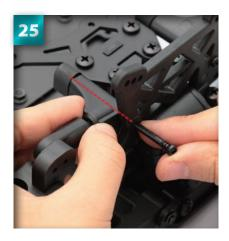
Tighten with a screwdriver, stopping as soon as the head of the screw rests against the shock stay.
