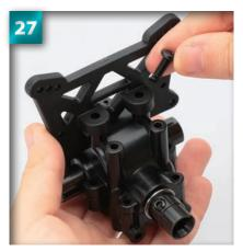
Tighten with a screwdriver, but as with the previous few steps, do not tighten too firmly.
