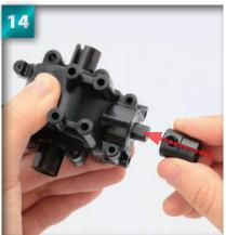
Slide the cup joint over the end of the driveshaft, as arrowed, with the hole on the cup joint facing upwards.
