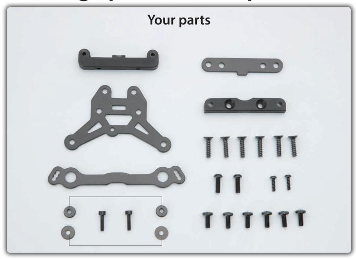
Front upper suspension holder Front lower suspension plate Front bulkhead plate Front lower suspension holder Steering plate
