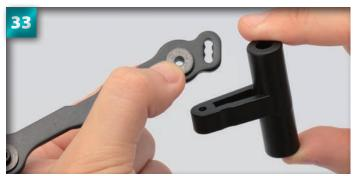
Holding the collar and washer in place, position the assembly onto the hole on the arm of the left servo saver. Make sure the servo saver is the right way up – the joint in the servo saver is on the bottom half of the body, below the arm.
