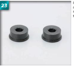
Inspect the steering collars on a flat surface. The wider ridge is situated at the lower portion of the collar.
