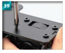
Repeat with the other three holes, again not tightening too hard. The heads of the screws should remain above the surface.
