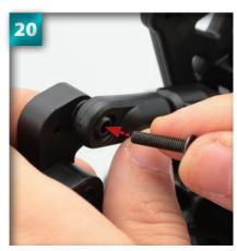
Holding the parts together, insert a 3 x 15mm countersunk screw into the hole in the ballshaped side of the flange ball (arrowed).
