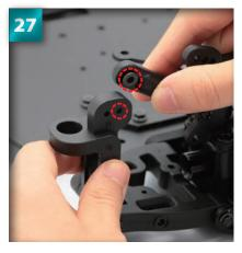
Line up the upper suspension arm's ball end and flange ball with the right front hub carrier. Make sure the hole in the flange ball is positioned against the circled hole on the hub carrier.
