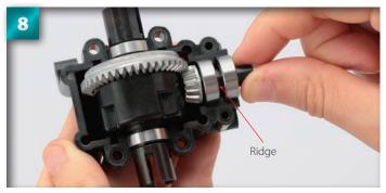
The driveshaft should sit so that the ridge in the recess separates the two ball bearings, and the teeth of the 13T bevel engage those of the 43T ring gear.
