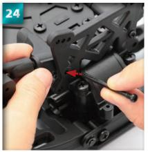
Hold the upper arm in place, and line up a 3 x 42mm screw shaft with the hole on the outside of the shock stay (arrowed).
