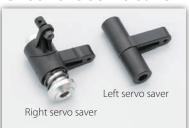
For this stage you will need the servo saver you assembled in Stage 3. Before beginning, check that the left and right are properly aligned.
