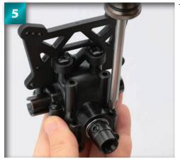
Tighten firmly with a screwdriver.
