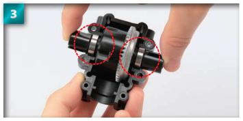
Your assembly should look like this, with the differential case sitting snugly into the lower bulkhead, and the right and left ball bearings resting in the cylindrical recesses on either side (circled).
