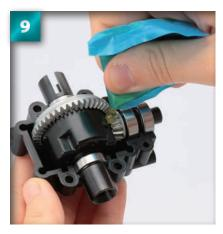
Apply some grease to the ring and bevel gears.
