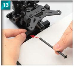
Insert the end of the suspension shaft into the hole on the bulkhead, following the red arrow. At this stage, just rest the tip of the shaft inside the hole – it should not protrude from the other side of the hole.
