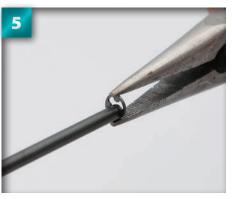
Use pliers to carefully clip one of the E-rings around the groove at the tip of the 4 x 74mm suspension shaft.
