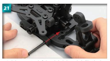
Push the suspension shaft through the holes on the bulkhead and suspension holder.
