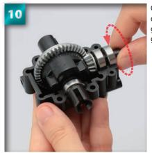
Gently rotate the driveshaft, so that the gears turn, spreading the grease evenly.
