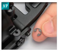
Line up another E-ring. It will fit onto the protruding tip of the shaft, with the open edge facing down and the rounded top side facing outwards.
