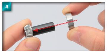
Slide one of the 1680 ball bearings over the driveshaft so that it rests against the back of the pre-fitted 13T bevel gear.
