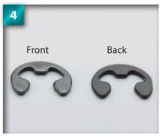
Now inspect the E3 E-rings, and make a note of which side is which - the front has rounded edges and the back is flat.
