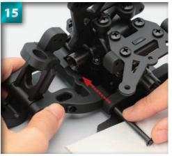
Once placed, push the suspension shaft right through the holes in the arms of the suspension holder so that it protrudes on the far side of the assembly.
