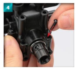
Now set one of the 3 x 10mm round-head screws into the hole on the bulkhead directly to the right of the cup joint.
