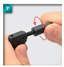
Turn the ball end so that it takes in the full-thread shaft. Keep going until about the same length of the thread that entered the upper arm (a little under half) is inside.
