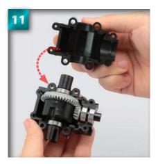
Make sure that the two parts are sitting flush with one another, and that they are not disturbing either of the ball bearings.
