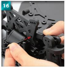
Hold the upper arm in place, and line up a 3 x 42mm screw shaft with the hole on the outside of the shock stay (arrowed).
