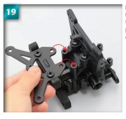
Lay the front bulkhead assembly flat on your work surface. Line up the holes on the front bulkhead plate with those on the bulkhead assembly (see arrows).
