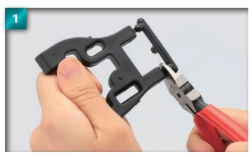
Use cutters to separate the front lower suspension arms from the remains of the plastic moulding.
