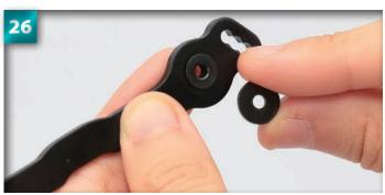
Still holding the collar from behind, place a 3 x 10mm washer over the front of the collar, as shown.
