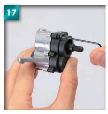
Using the 1.5mm Allen key, tighten a 2 x 10mm cap screw into the first of the holes.
