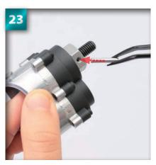
Make sure that both ends of the pin are sitting flush to the side of the wheel hub.
