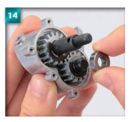
Grease the tip of the reduction shaft, then slide on the 1260 metal bush.
