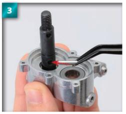
Grease the base of the reduction shaft, then use tweezers to insert the 2.5 x 12mm pin through the hole arrowed.
