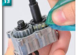
Apply a little grease to both gears.
