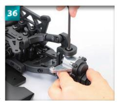
Tighten with the 3mm Allen key.
