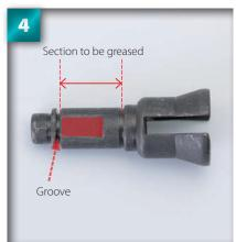
Inspect the front reduction shaft – on either side of the thinner section of the part there are flat sections (highlighted). There is also a narrow groove set around the tip of the shaft (arrow).
