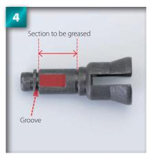
Inspect the front reduction shaft – on either side of the thinner section of the part there are flat section (highlighted). There is also a narrow groove near the end of the shaft (arrowed).
