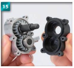
To close the hub, line up the front right hub outside with the assembly produced in this session. The wheel reduction shaft will fit through the hole in the hub outside, and the six screw holes should meet.
