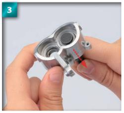
Pull the wheel reduction shaft and bush through the bottom hole of the front left hub inside, from the angle shown in the photograph.
