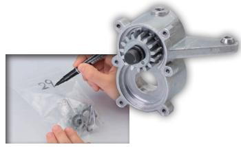
This is only a temporary assembly, so keep all the parts in a plastic bag for later use, preferably sealing with cellophane tape to prevent any parts falling out. It is a good idea to mark the stage number on the plastic bag for future reference.
