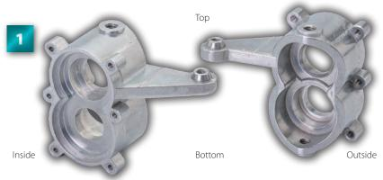
Familiarise yourself with the front left hub inside. The 'knuckle arm' is the triangular section that protrudes from just above the middle of the hub's body. Also, make a note from the photo of which is the inside and outside of this part.
