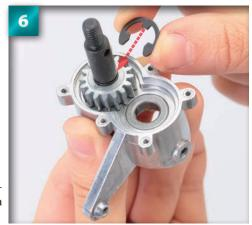
Fit the E7 E-ring around the groove in the wheel reduction shaft (see arrow), with its rounded side facing up. Make sure you use the E7 E-ring the smaller E6 E-ring will be used in a later step.
