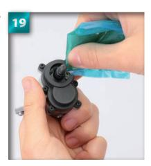
Slide the 1680 metal bush over the wheel shaft and into the recess. Turn back and forth to spread the grease evenly inside.
