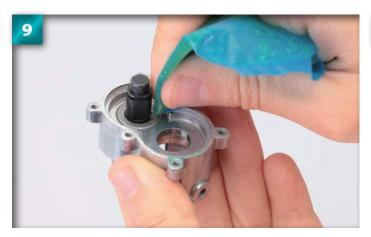
Apply a little more grease to the protruding section of the reduction shaft.
