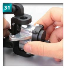
Make a note of the shape of the knuckle collars – the outside has a wide, flat surface, while the inside is smaller and rounded.
