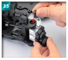
Insert a 4 x 10mm cap screw through the hole in the knuckle collar and into the hole in the top part of the hub.
