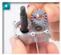
Make sure equal parts of the pin are visible on either side of the shaft, then slide on the 16T reduction gear, back side first. The grooves on the back of the gear should accommodate the tips of the pin (see circles).
