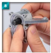
Hold the bush in place to stop it slipping, then turn the reduction shaft back and forth to spread the grease.
