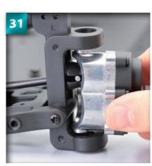
Make a note of the shape of the knuckle collars – the outside has a wide, flat surface, while the inside is smaller and rounded.
