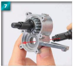
Re-insert the reduction shaft you removed in Step 1. Once in place, apply some grease to the protruding end of the shaft.
