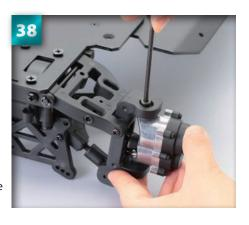
Tighten the cap screw into place with the 3mm Allen key.
