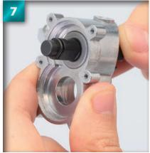
Turn the reduction shaft back and forth to spread the grease.
