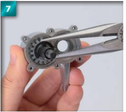
Clip the E-ring into place with pliers, making sure that the flat back of the E-ring is touching the gear, and the rounded front is facing upwards.
