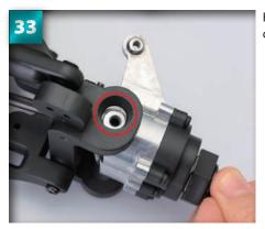
Hold the hub assembly in place, and check that the holes are aligned.
