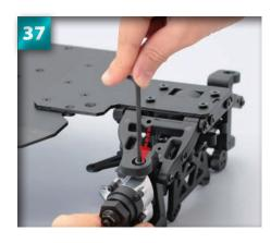
Holding the hub in place, turn the assembly over so that you have access to the underside of the suspension system. Place the second knuckle collar into the hole in the bottom side of the hub carrier; then, as you did in Step 36, tighten into place with the second 4 x 10mm cap screw, using the 3mm Allen key.
