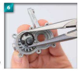
Use pliers to carefully clip the E-ring around the groove.
