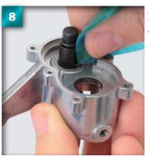
Apply a little more grease to the protruding section of the reduction shaft.
