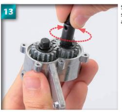
Slowly rotate the wheel reduction shaft to spread the grease evenly across the gears.
