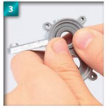
Evenly press the bush into place using both thumbs. It is important to push straight, as even a small angle will block the part. Do not force it, as this may damage the bush and cause problems at a later stage.
