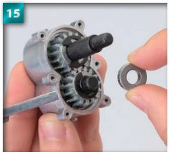
Apply a little grease to the tip of the reduction shaft, then slide the 1260 metal bush over it, so that it sits on top of the E-ring.
