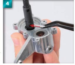
Turn the assembly over, and insert the 2.5 x 12mm pin through the hole in the wheel reduction shaft. Using tweezers will make this easier.
