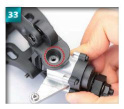
Hold the hub assembly in place, and check that the holes are aligned.
