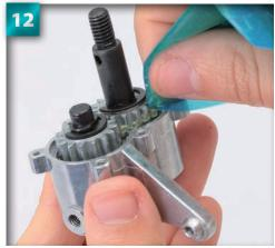
Apply a good amount of grease to both gears.
