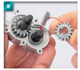
Slide the 15T reduction gear over the shaft, so that it rests on top of the greased bush, with its teeth engaging those of the 16T gear.
