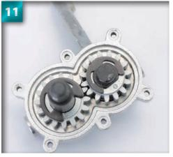
Your assembly should look like this, with the gears interlocked neatly.
