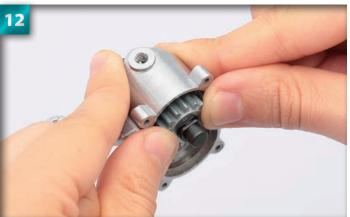
Push the gear firmly into place so that the thin groove near the tip of the reduction shaft (labelled in Step 4) is visible above the surface of the gear.
