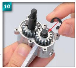
Place the E6 E-ring around the groove in the tip of the reduction shaft, with the rounded top side of the E-ring facing upwards.
