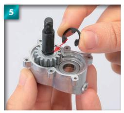
Position the E7 E-ring around the thin groove in the shaft, just above the surface of the gear. The rounded side of the E-ring should be facing upwards. Be sure to use the E7 E-ring – the smaller E6 E-ring will be used in a later step.
