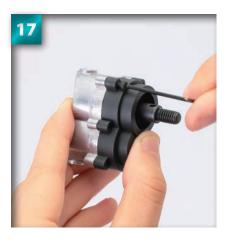
Insert a 2 x 10mm cap screw into one of the holes on the hub outside and tighten with the 1.5mm Allen key.
