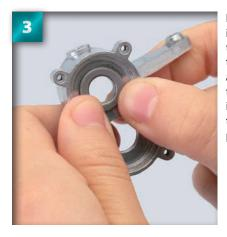
Evenly press the bush into place using both thumbs. It is important to push straight, as even a small angle will block the part. Do not force it, as this may damage the bush and cause problems at a later stage.
