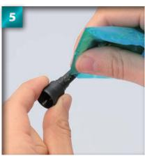
Insert the reduction shaft through the top hole of the hub, entering from the outside (the shaft will go through the metal bush on the inside).
