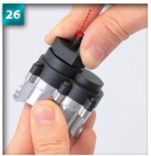
Press down firmly on the adaptor so that it conceals the wheel hub inside completely.
