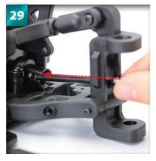
Position the chassis assembly on your work surface, so that the front right suspension system is easily accessed. Insert the front right driveshaft through the gap in the hub carrier, then slot its head into the differential cup joint, as shown.
