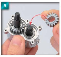
Slide on the 15T gear, back side first. The teeth should interlock with those of the 16T gear when level.
