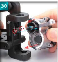
Hold the other end of the driveshaft level, and position the cup joint at the back of the hub so that it accommodates the head of the driveshaft. Line up the circled pins with the slots on the joint.
