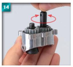
Rotate the wheel reduction shaft to evenly disperse the grease.
