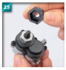
Cover the wheel hub with the wheel hub adaptor.
