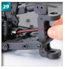
Position the chassis assembly on your work surface, so that the front left suspension system is facing you. Insert the front left driveshaft through the gap in the hub carrier, then slot its head into the differential cup joint, as shown.
