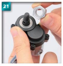
Slide the wheel hub over the wheel shaft, so that the side with the raised circle (see photo) sits on top of the bush.
