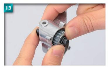
Push the gear firmly into place so that the thin groove at the tip of the reduction shaft (labelled in Step 4) is visible above the front surface of the gear.
