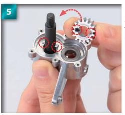
Make sure that equal parts of the pin are visible on either side of the shaft, then slide on the 16T reduction gear. The tips of the pin should sit inside the grooves in the back of the gear (see circles).
