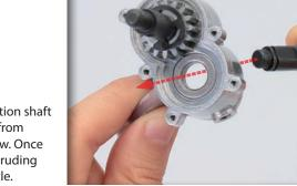
Now re-insert the reduction shaft you removed in Step 1, from the direction of the arrow. Once in place, grease the protruding section of the shaft a little.
