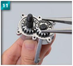
Your assembly should look like this. Make sure the teeth of the gears are interlocked, and the rounded top sides of the E-rings are facing upwards.
