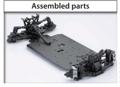
This stage is now complete. Your Hummer has its front and back suspension systems and all four wheel hubs installed, ready for the next stages. Store your assembly away safely until next time.
