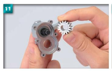
The reduction gear will fit over the tip of the reduction shaft back side first.
