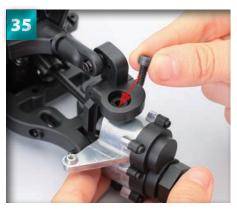
Insert a 4 x 10mm cap screw through the hole in the knuckle collar and into the hole in the top part of the hub.
