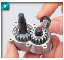
As you did with the E7 E-ring in Step 5, position the E6 E-ring around the thin groove in the reduction shaft. Again, the side with rounded edges should face upwards.
