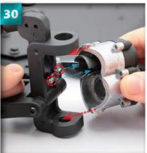
Hold the other end of the driveshaft level, and position the cup joint at the back of the hub so that it accommodates the head of the driveshaft. Line up the circled pins with the slots on the cup joint.
