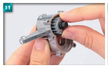
Line up the gear so that the flat sections accommodate those on either side of the reduction shaft.
