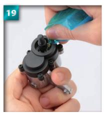
Slide the 1680 metal bush over the shaft and into the recess. Turn from left to right a few times to spread the grease.
