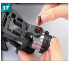
Holding the hub in place, turn the chassis assembly upside down to gain access to the underside of the hub carrier. Repeat Steps 33 to 35 for the set of holes on this side.
