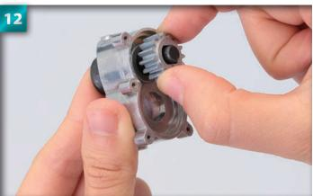
Line up the gear so that the flat sections of the hole in the middle fit against the corresponding flat portions on either side of the reduction shaft.
