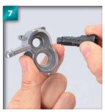
Insert the reduction shaft through the top hole of the hub, entering from the outside (the shaft will go through the metal bush on the inside).
