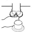
10. Connect rubber joints to both ends of the inlet hose.
