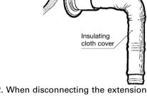
When disconnecting the extension pipe (such as flexible pipe and flexible elbow), pull the pipe by turning the pipe clockwise.
