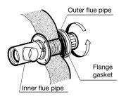
7. Insert the flexible exhaust pipe to the flexible bent joint until it locks. Insert the flexible bent joint to the exhaust mouth of the inner flue pipe until it locks.
