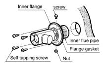
Install the flange gasket to the outer flue pipe. Secure
