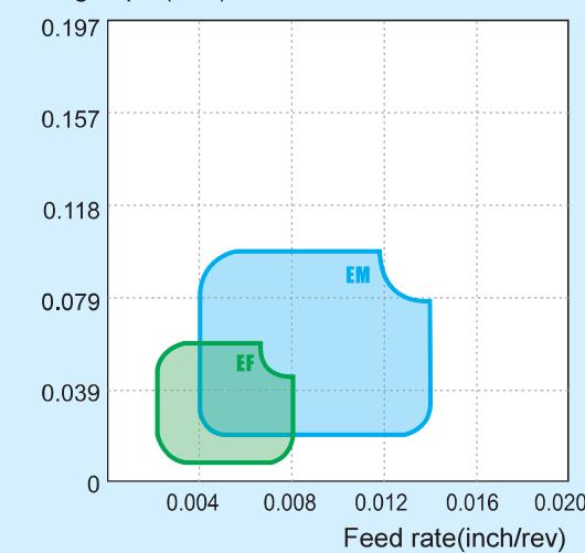
► Workpiece material: stainless steel (Austenitic 321)
