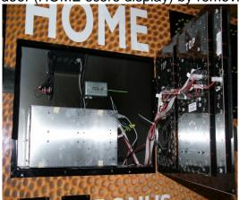
1. Inside the scoreboard, connect the control cable leads to the appropriate terminals on the terminal block, according to the label above the terminal block.
