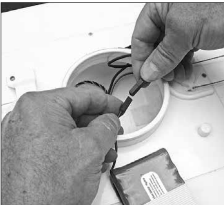
Step 10. Connect the battery pack. Time: 10 sec.
