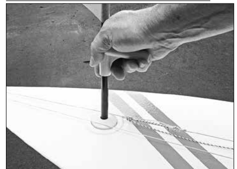
Step 6. Drop mast with sail into mast step. Time: 5 sec.
