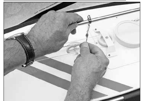
Step 9. Attach sheet line to boom clip. Time: 5 sec.
