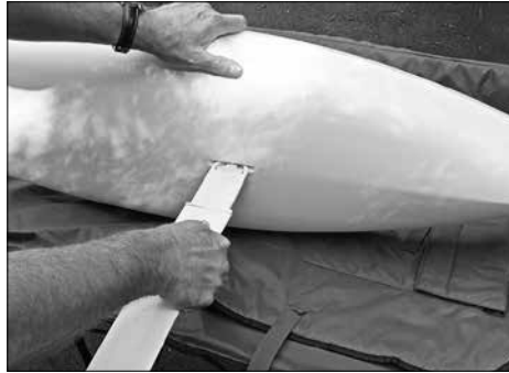
Step 2. Insert keel into slot, turn toggle. Time: 10 sec.
