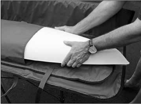
Step 1. Unzip carry bag, remove boat hull. Time: 10 sec.
