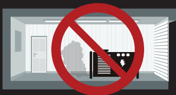
Running a generator indoors or too close to a living area
