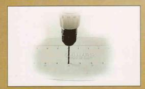
STEP 1 Select and drill through pre-punched number holes using drill bit provided with address plaque
