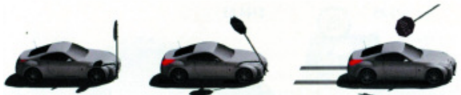
High speed VR3 / VR4 anchor impact
