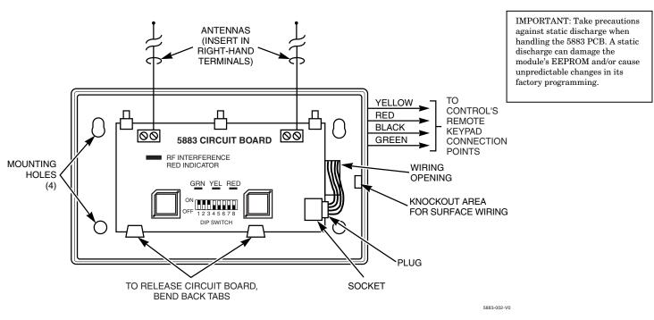
Figure 5. 5883H RF Transceiver
