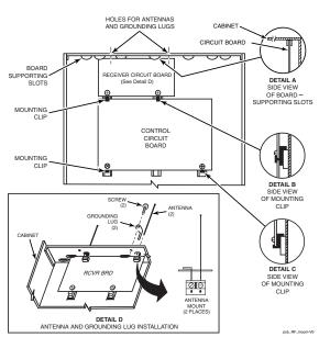
Figure 2. Installing the 5883H Board in the Control's Cabinet (Check the control's Installation Instructions for applicability.)
