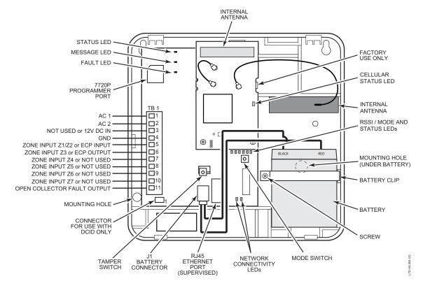
NOTE: All circuits are supervised and all circuits are power limited except the battery.
