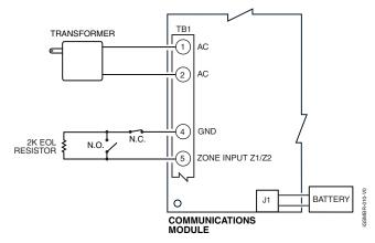
Wiring Zone 1 Input for EOL Supervised N.O. /N.C. Triggers
