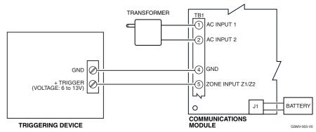
Wiring Zone 1 Input for a Positive (+) Trigger
