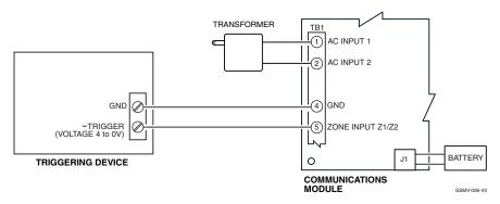
Wiring Zone 1 Input for a Ground (-V) Trigger
