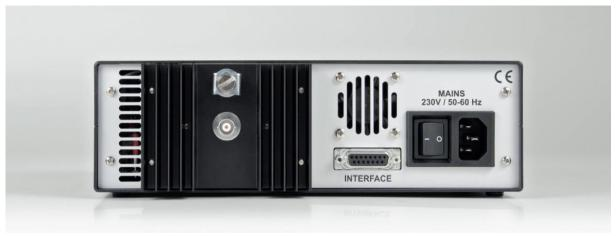
Converter negative connection: Shield of the BNC socket Converter positive connection: Inner conductor of the BNC socket
