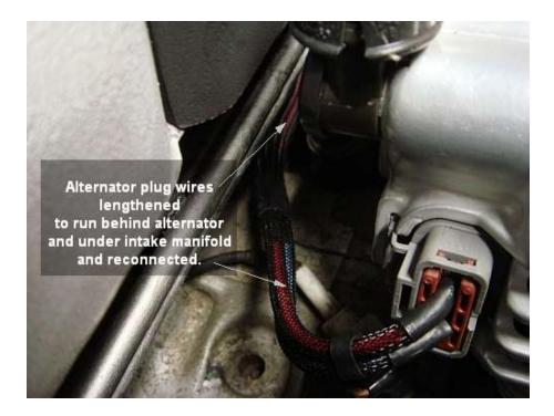
The same lengthening procedure was done to the two small A/C connector wires, which entered the plastic channel by the A/C compressor. These run under the intake manifold as well and are also protected with the same heat-resistant braided sleeving. They are hidden out of sight for a clean look.
