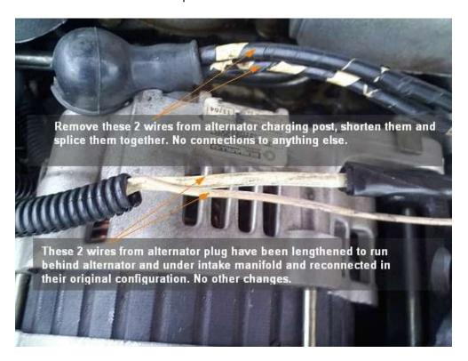
The alternator plug wires were removed from the plastic channel and cut. Be sure to remember which wires are which when you add an additional length of wire to each. You can do this by doing one wire at a time. Using a longer length of wire allows you to run the wires behind the alternator and under the intake manifold and be reconnected at their original position by the battery. These wires were soldered and shrink-wrapped and encased in heat-resistant nylon expandable braided sleeving.
