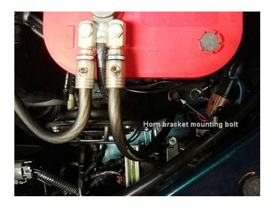
I used a different type of connector, **4 gauge StreetWires Power Rings**, for these wires to increase electrical conductivity, as well as provide a stronger connection. Just one connection at the battery post to totally disconnect power.
