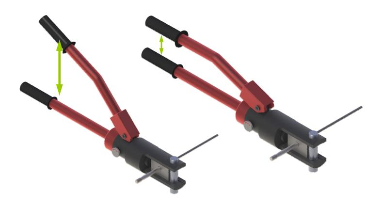
8. Reposition the dies 1/4" further along the fitting and rotate 45 degrees. Repeat the crimping process for a total of three crimps.
