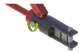
5. Position the jaws around the fitting, 1/8" from where the cable enters the fitting.
