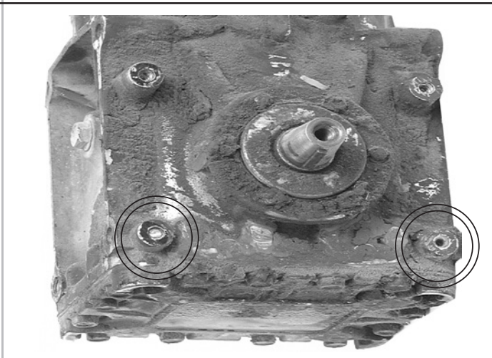
Stripped, broken or damaged clutch mounting threads.
