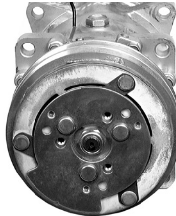
Extreme heat build-up causing clutch failure, due to slipping, lack of lubrication or high system head pressure.
