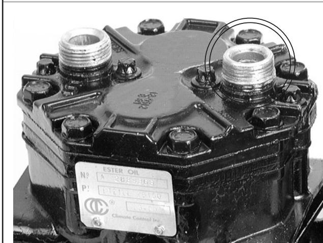
Stripped Fitting due to overtightening service valve.
