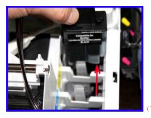
Step 5: When the inner cartridges have been fitted, the direction of tube can be fixed according to the USB groove as picture 8 & 9 shown.
