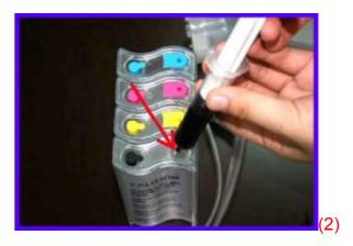
Step 2: Open the stopper of the inner cartridge as picture 3 shown; then insert the filling tool to the hole as the picture 4 shown.
