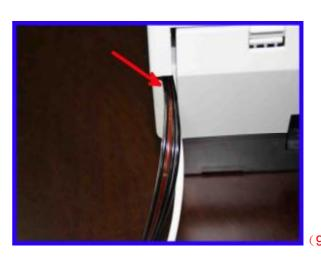
Step 6: Please do not press the tube of Continuous Ink system when closing the cover of printer, Then insert the stopper of the ink filling hole back to ink tank and open the small stopper of air hole on Ink tank.. Then print the test paper to have a test.
