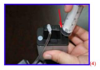
Step 3: Draw out the handle of filling tool; then ink will slowly flow into the inner cartridge as picture 5 shown; stop pulling the handle when the inner cartridge is full of lnk. Then put the stopper back to inner cartridge.
