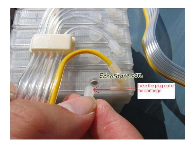
5. When the cartridge is full, put the plug back. Please be careful so that the ink will not be out of the cartridge.
