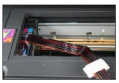
Stimulate the move of the cartridge car. Insure there will no block and when the tubes moving with cartridge car.
