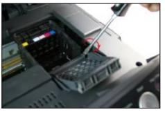
Use a screwdriver to insert into the joint slightly
