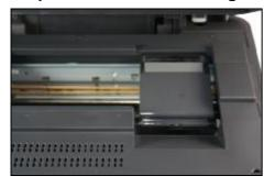
Remove the clip of the carriage, then you can get the cartridge out..
