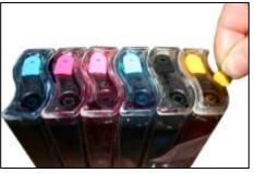
Pull out the small rubber plug from the air hole on each inktank.
