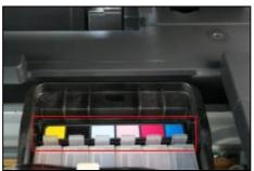
Place the CIS cartridge according to the color label
