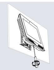
5. REMOVE PANEL FROM MOUNT: With two hands low on the panel, carefully apply pressure to the panel bottom outward to separate the panel from the mounting plate attached to the wall.
