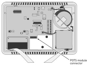
2 Match the 7 x2 pin set and the 2 white mounting clips on the back of the POTS Module to the open pin set and 2 holes on the back of the Control Panel.
