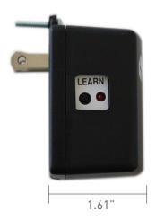
NOTE: The Universal Garage Door Receiver (2GIG-GDR1-345) is designed to work with the new 4-Button Key Ring Remote (2GIG-KEY2-345) and will not work properly with the 4-Button Key Ring Remote (2GIG-KEY1-345)
