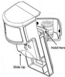
Figure 4. Removing Sensor for Battery Replacement
