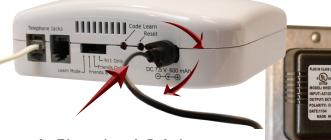
A. Plug the AC Adapter power cord into the power jack and twist 1/4 turn clockwise to lock. B. Plug the AC Adapter into an electrical outlet.
