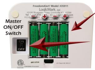
1A. Place the Green AA Rechargeable Batteries in the compartment on the bottom of the base unit. Check the picture for correct orientation.
