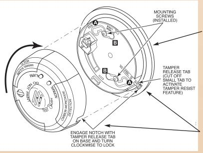
A sturdy mounting base allows the detector to be flushmounted to walls, to smooth and uneven ceilings (i.e. stucco).
