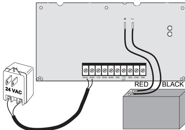
3. Wire the power supply AC transformer to the power supply board, then plug in the transformer (Figure 10). The green LED should turn on to indicate power is present. The red LED should be off for the moment.
