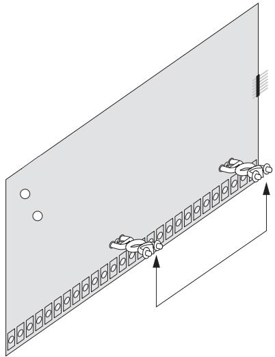
3. Slide the top of the backplates onto the left and center module mounting clips on the panel cabinet (Figure 4), then snap the backplates on to the support standoffs (Detail in Figure 4).
