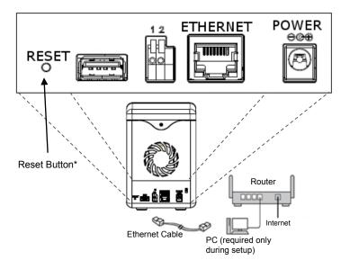
\*If you experience difficulties with the camera setup process, hold down the reset button for 15 seconds to reset the SVR.
