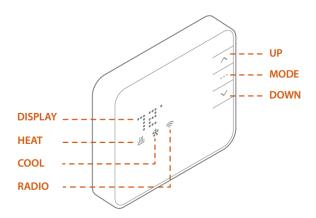
1. Press any button to wake the thermostat up.
