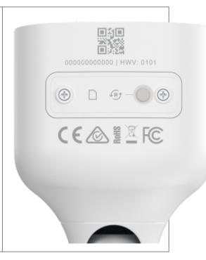
**Important**: Once a video device has been reset, it is normal for the LED to turn off momentarily. It is best to leave the video device plugged into power and undisturbed for two minutes after performing the factory reset.
