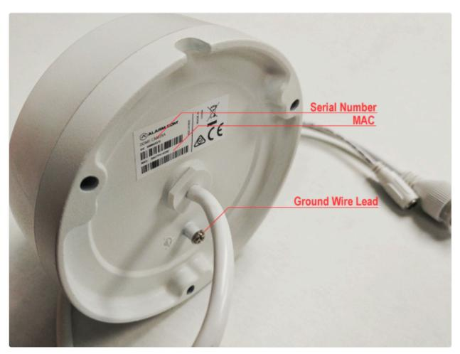
The following image displays the sticker found on a video device's box. The firmware version that was initially loaded on the camera is also located on the box sticker as *FW*.
