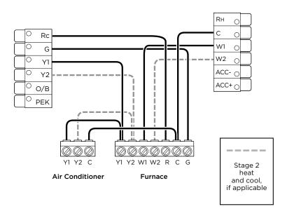
NOTE Do not connect any jumper wires between Rc and Rh. ecobee does this automatically. The R wire needs to go into the Rc terminal on your ecobee.
