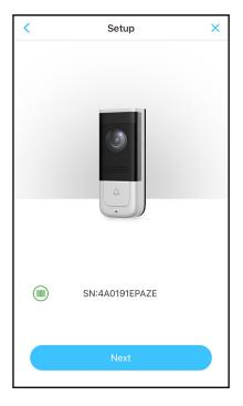
6. Enable your doorbell "hotspot": With the doorbell LED flashing (indicating it is not yet connected to a network), press and release the "Reset" button located on the back of your doorbell (see diagram on page 7). The doorbell will beep 3 times and its LED will begin to scroll. Tap Next.
