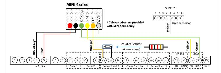
Wiring the MiNi Series with Ringer MN01-RNGR to Honeywell Vista 15P/ 20P for UDL
