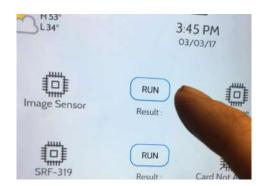
Run the "Image Sensor" test. Allow up to 2 min for the panel to successfully test the radio in the new IQ Card-IS. If test fails, reboot the panel and try again.
