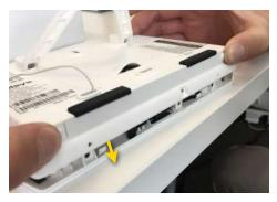
Replace the back cover, taking care not to pinch any antennas or wires.
