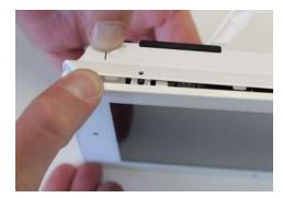
Push down on the two tabs located on the bottom of the panel and pull the panel away from the back plate
