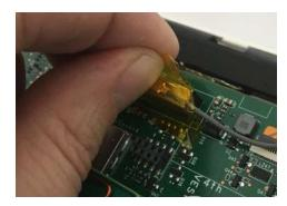
Remove the tape holding the end of the antenna to the board
