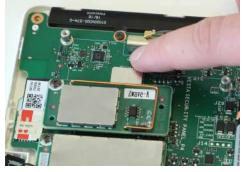
Locate the free space above the Z-Wave radio
