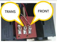
The Adapter leads wire to the doorbell chime's TRANS and FRONT terminals inside the house.
