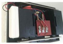
Use the supplied double sided adhesive tape to mount the IQ Doorbell on the doorbell chime. Make sure to put it in an area that still allows for the decorative cover to be replaced.
